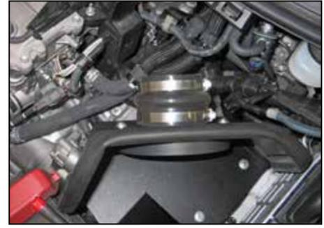
21. Install the provided silicone hose (087121) onto the filter adapter as shown.
