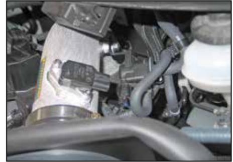
23. Secure the EVAP solenoid bracket to the intake tube with the provided hardware.
