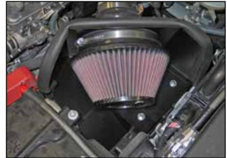
25. Install the K&N® air filter onto the filter adapter and secure with the provided hose clamp.
