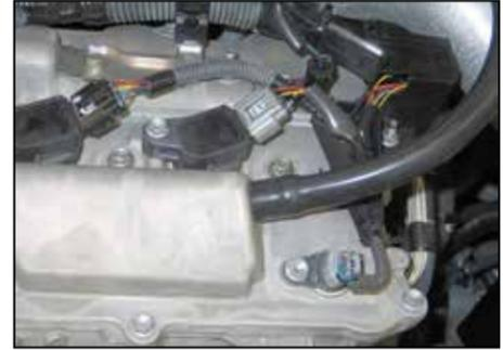
24. Connect the crank case vent hose to the valve cover port.
