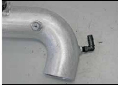
18. Install the 90° vent fitting into the K&N® intake tube as shown.
