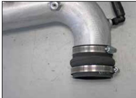
20. Install the provided silicone hose (087121) onto the throttle body end of the K&N® intake tube as shown.
