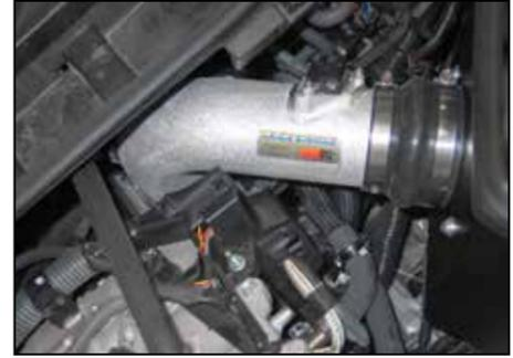
22. Install the K&N® intake tube assembly onto the throttle body and filter adapter, then secure with the provided hose clamps.
