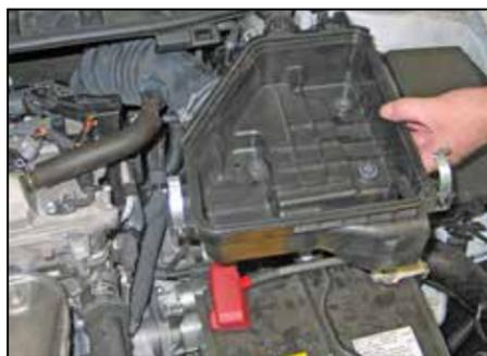
6. Unhook the fresh air duct from the lower air box, unhook the engine wiring harness from the rear of the air box and then remove the lower air box from the vehicle.
