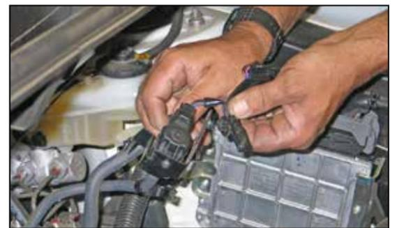
8. Un-hook the EVAP wiring harness from the EVAP mounting bracket as shown.
