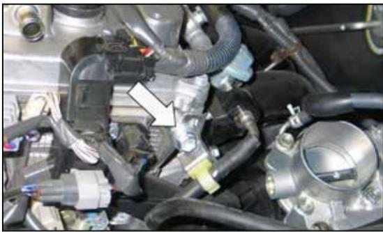
10. Remove the fuel rail mounting bolt shown.
