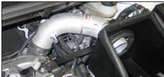
19. Install the intake tube into the silicone hose at the throttle body and align with the mounting bracket. Secure the EVAP bracket and mounting bracket in the same location on the intake tube using the provided hardware.
