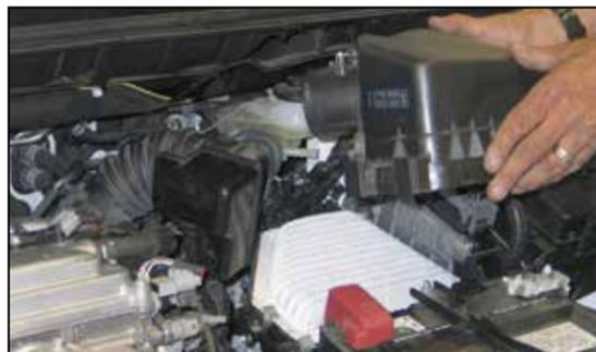
5. Loosen the hose clamp that secures the intake tube to the upper air box. Then, un-hook the three upper air box retaining clips. Remove the upper air box from the vehicle as shown.
