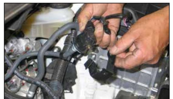
9. Remove the screw that secures the EVAP mounting bracket, then remove the bracket as shown.
