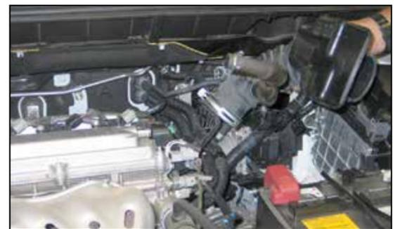
7. Disconnect the crank case vent hose from the valve cover. Loosen the spring clamp that secures the intake tube to the throttle body and remove the stock intake tube from the vehicle.
