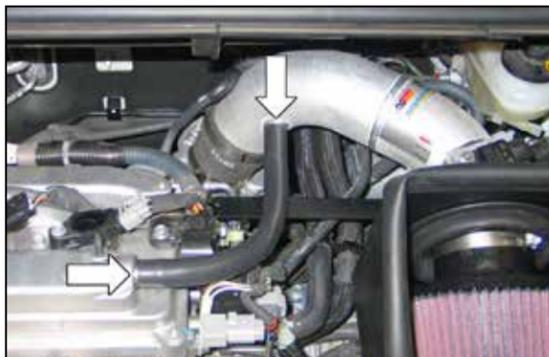
21. Install the provided crank case vent hose as shown.
