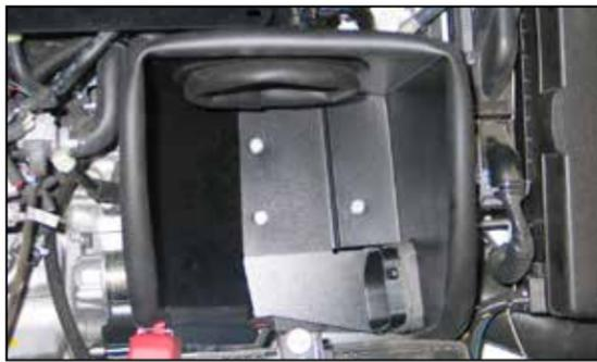
16. Install the heat shield assembly and secure with the provided hardware.
