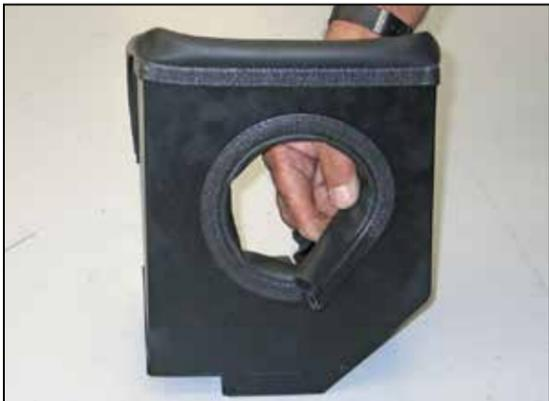
15. Install the short edge trim onto the heat shield as shown.
