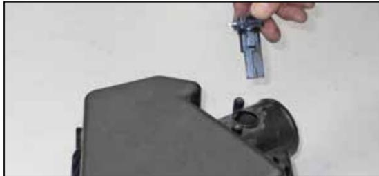
17. Remove the two screws that secure the mass air sensor to the stock air box. Then, remove the mass air sensor as shown.
