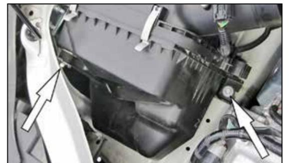
8. Remove the bolt and nut that secure the air filter housing into the vehicle and then remove the air filter housing from the vehicle.
