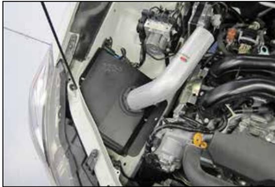
17. Install the intake tube/heat shield assembly into the engine compartment as shown and connect the mass air sensor connection, then secure the heat shield with the provided hardware and factory nuts from step 8.
