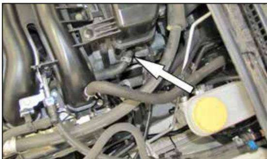
2. Release the spring clamp securing the crank case vent hose to the intake plenum and then disconnect the hose from the plenum.
