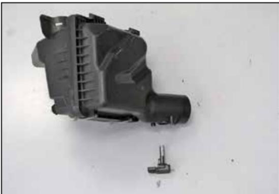
12. Remove the two screws securing the mass air sensor to the factory air filter housing and then remove the sensor from the housing.
