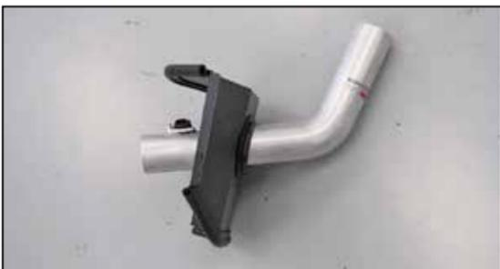
15. Pass the intake tube assembly through the heat shield and secure it to the bracket with the provided hardware.
