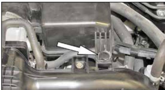
3. Remove the plastic clip which secures the intake plenum to the intake manifold.
