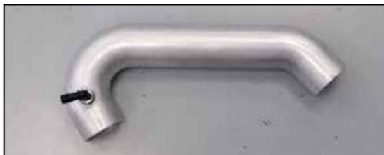
19. Install the 90° NPT vent fitting into the K&N® intake tube as shown.
