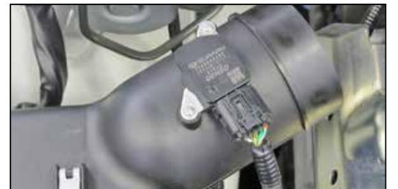
7. Disconnect the mass air sensor electrical connection.
