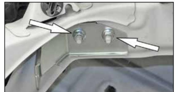
9. Remove the two nuts that secure the air filter housing bracket onto the inner fender. **NOTE: These nuts will be reused in a later step.**
