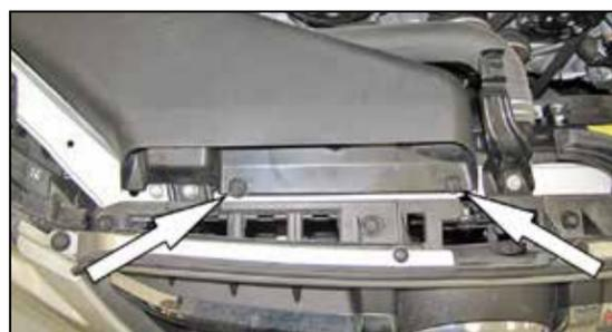
6. Remove the two plastic clips securing the intake scoop to the core support and then remove the intake scoop from the vehicle.
