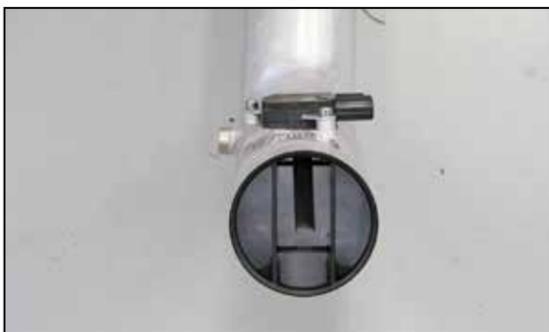
14. Place four drops of the provided super glue onto the lip of the provided air grid and then install the air grid into the K&N® intake tube as shown.
