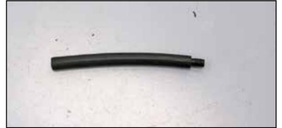
22. Install the provided hose mender into the provided crank case vent hose as shown.
