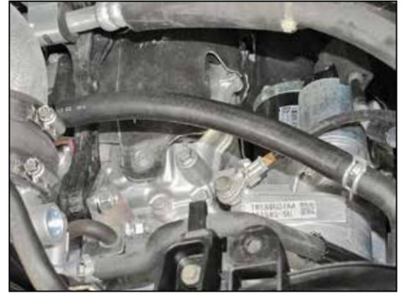
23. Install the open end of the hose mender into the factory crank case vent hose and then connect the hose to the fitting installed into the K&N® intake tube.
