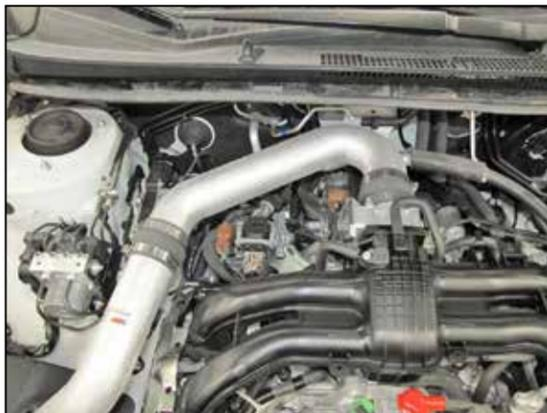
21. Install the remaining coupling hose onto the intake tube and install the intake tube into the hoses and adjust the tubes for best fit. Then secure the provided hose clamps.
