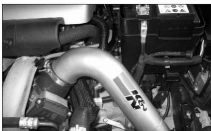
26. Fit the K&N Typhoon intake tube into the silicone hose using the #44 hose clamp supplied. (Do not fully tighten yet!) **NOTE: always clean the inside of the tube first.**
