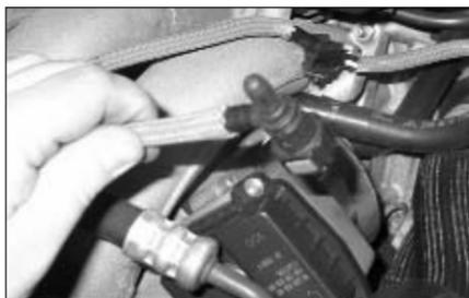
9. Remove the small vacuum hose and fit a rubber tip supplied onto the connector as shown. Re-install the connector to the intake manifold.
