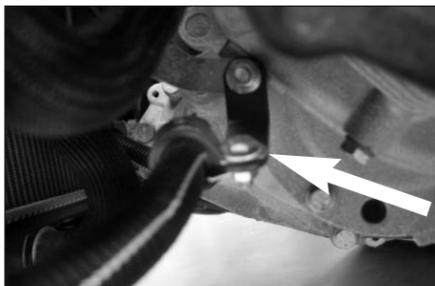
22. Fit the "P" cable clamp supplied around the wiring loom and mount it onto the bracket using the M5 allen head bolt, nut and washer supplied.
