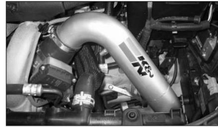
33. Align the intake tube for best fit and clearance, then, firmly tighten the hose clamp and M6 bolt and M6 nut. To provide more clearance between the filter and the arch liner you can insert the tube further into the silicone hose of the throttle body.
