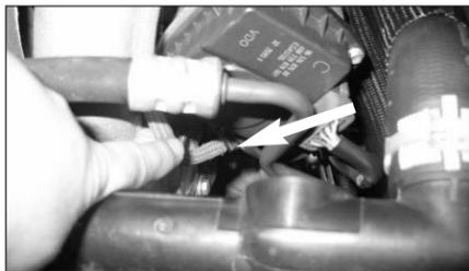
8. Remove the vacuum connector from the intake manifold. (This is the gray one.)
