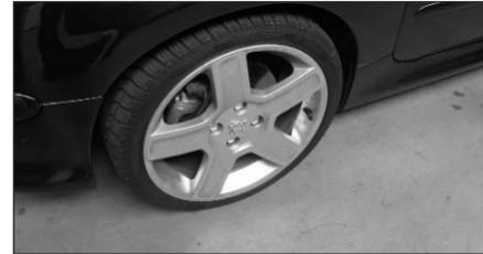
31. Refit the wheel arch liner and the wheel to the vehicle. Torque the wheel up to factory specifications.
