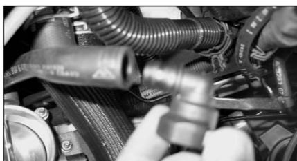
11. Remove the elbow connector from the breather hose from step 2.
