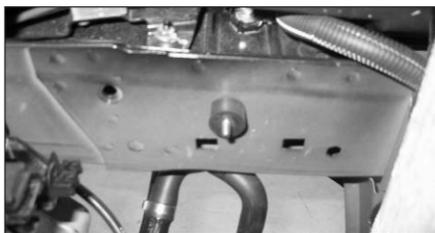
23. Screw the rubber vibration stud onto the air box mounting point from step 5 as shown.
