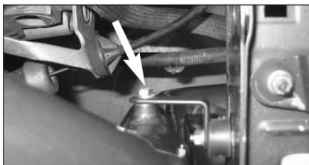
27. Fit the tube on the rubber mounting stud as shown and secure with a M6 nylock nut and M6 washer supplied. Do not fully tighten yet!
