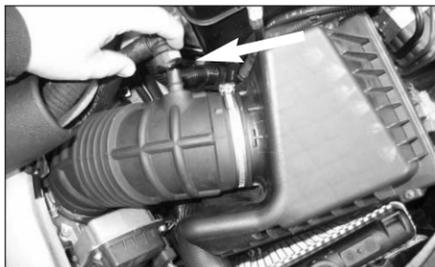
2. Remove the breather hose from the intake tube as shown. Release the 2 hose clamps and remove the intake tube from between the air box and the throttle body.
