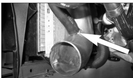
28. Fit the air pump hose onto the vent on the intake tube as shown. It may be necessary to trim the hose for better fitment.
