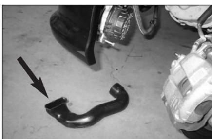
19. Unclip and remove the cold air intake tube from the vehicle.
