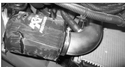
30. Fit the Drycharger over the filter as shown. **NOTE:** The Drycharger's water repellant properties will last up to two years. See the parts list to re-order Drycharger if necessary.
