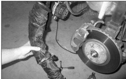
18. Unclip and remove the cold air intake tube located in the wheel arch from the vehicle.
