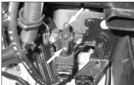
10. Fit two rubber tips supplied onto the electronic vacuum switch from step 7 as shown.
