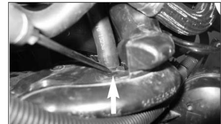
14. Carefully unclip and remove the air pump hose from the resonator box as shown.
