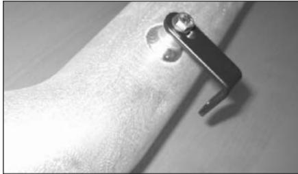
24. Fit the L bracket onto the intake tube using the M6 bolt, M6 waved washer and M6 washer supplied. Do not fully tighten yet!
