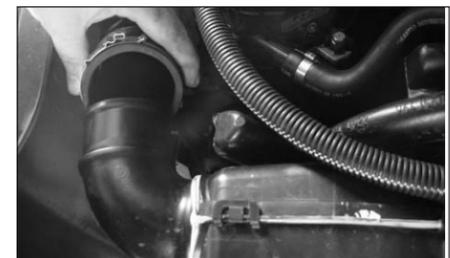
13. Unclip the intake snorkel from the resonator box.
