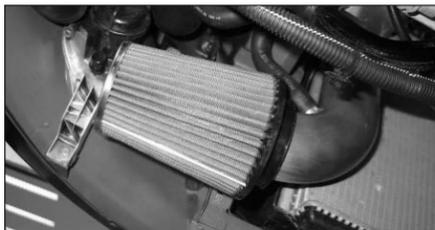
29. Fit the filter onto the K&N Typhoon intake tube using the #44 hose clamp supplied.
