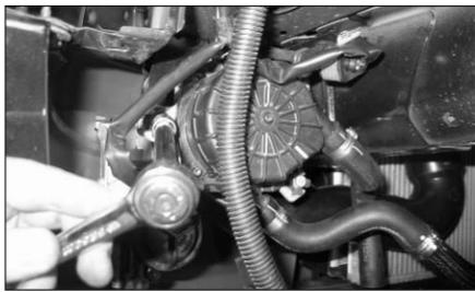
17. Remove the bolts securing the air pump to the vehicle, so that the air pump can be moved out of the way.
