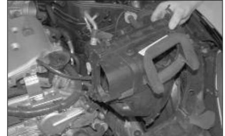
9. Pull firmly upwards to release the air cleaner base from the factory grommets, then remove the air cleaner base as shown. **NOTE: K&N Engineering, Inc., recommends that customers do not discard factory air intake.**
