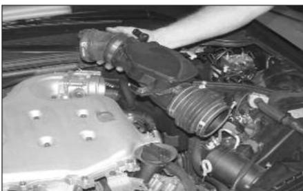
5. Remove the stock intake tube as shown.
