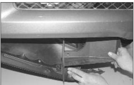
16. Remove the plastic cover from the styrofoam block off panel from step 15 and reinsert the plastic cover onto the radiator core support and secure it with the plastic rivets.
