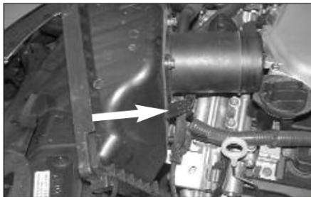
7. Unclip the air cleaner lid, then, loosen and remove the single bolt that secures the air cleaner lid to the fender. Rotate the air cleaner lid, then, unclip the mass air sensor electrical connection to remove the air cleaner lid as shown.
