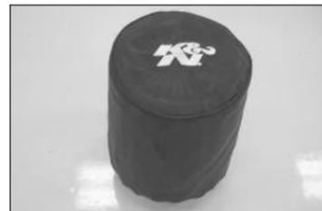
29. Install the provided K&N® Drycharger® onto the K&N air filter as shown. **NOTE:** The Drychargers water repellent properties will last up to two years. See the parts list to reorder a new Drycharger if necessary.
