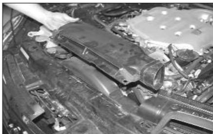
8. Disengage the two plastic rivets, then, remove the stock air inlet duct as shown.
