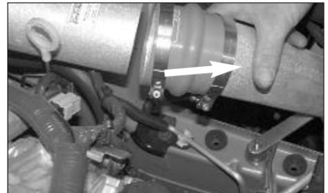
26. Install the K&N® Typhoon® cold air tube into the vehicle and line up the bracket with the rubber mounted stud as shown.
