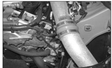
27. Slide the silicone hose over the short ram tube as shown.
