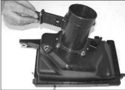
17. Loosen and remove the two screws to remove the mass air sensor from the stock air cleaner lid as shown.
