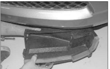
15. Remove the styrofoam/plastic block off panel as shown.
