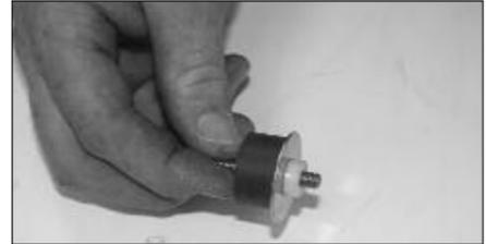
23. Install the fender washer and nylon washer onto the rubber mounted stud as shown.
