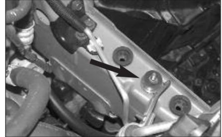
24. Install the rubber mounted stud assembly into the threaded hole from step 23 as shown.
