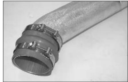
25. Slide the silicone hose and hose clamps onto the K&N® Typhoon® cold air tube as shown.
