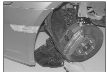
11. Remove the nine bolts and six plastic rivets, then, lower the inner fender valance down as shown.
