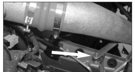
28. Secure the bracket to the rubber mounted stud using the provided hardware as shown, but do not tighten completely at this time.
