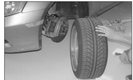
10. Raise the vehicle up and support it with jack stands, then, remove the front driver side tire as shown.
