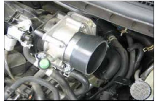
23. Install the provided silicone hose (08440) onto the throttle body and secure with the provided hose clamp.
