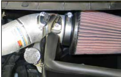
31. Reconnect the mass air sensor electrical connection.
