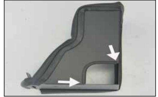
21. Install the provided edge trim into the heat shield fresh air duct opening as shown.
