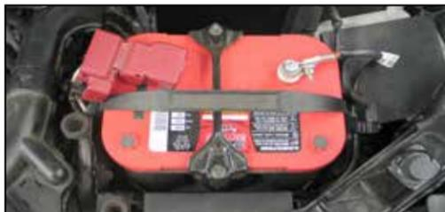
35. Reinstall the battery and secure with the factory hold down. Reconnect the positive and then the negative battery cables.
