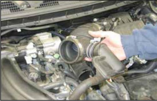
9. Remove the intake hose assembly.
