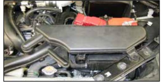
36. Reinstall the intake resonator onto the fresh air intake duct.
