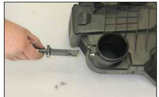
24. Remove the screws securing the mass air sensor and then remove the mass air sensor from the stock air box.
