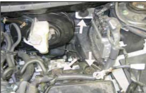
12. Remove the three air box mounting grommets shown from the air box mounts.
