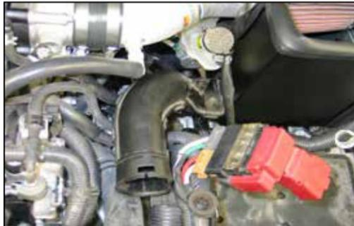
33. Install the lower fresh air duct into the heat shield as shown.
