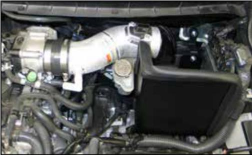
28. Install the K&N® intake tube into the silicone hose at the throttle body and align with the tube mounting bracket. Secure the intake tube with the hose clamp and hardware provided.
