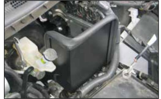
22. Set the heat shield into position on the mounting bracket and rubber mounted studs then adjust as necessary. Secure the heat shield and bracket with the provided hardware.
