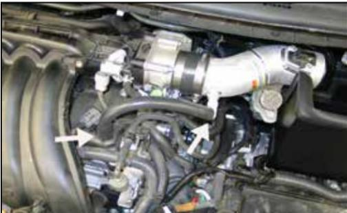
29. Install the provided silicone hose onto the crank case vent port on the valve cover and then attach the other end to the 90° fitting installed in the K&N® intake tube.
