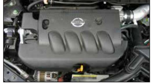
37. Reinstall the engine cover and secure with the factory mounting bolts.
