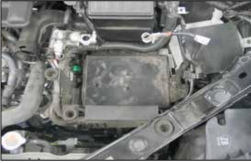
7. Remove the positive battery cable and battery mounting bracket, then remove the battery from the vehicle.
