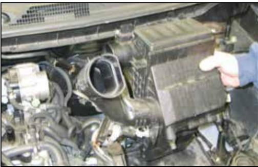
11. Lift up the air box to dislodge it from the mounting grommets and then remove the air box from the vehicle.
