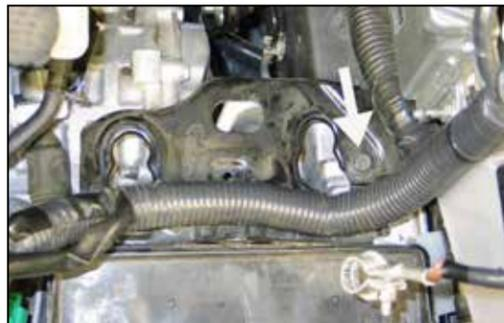
18. Remove the air box mounting plate bolt shown.
