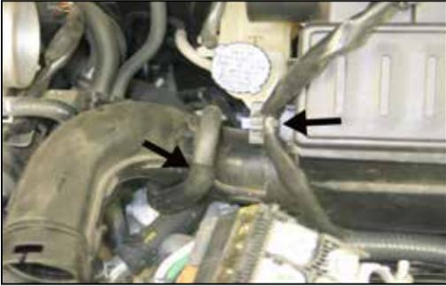
10. Disconnect the transmission vent line and wiring harness from the air box.
