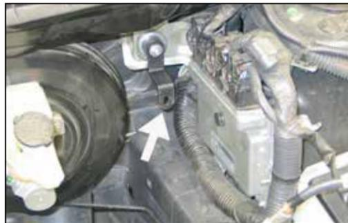
16. Install the provided bracket (010033) onto the rubber mounted stud installed in step #16 and secure with the provided hardware.
