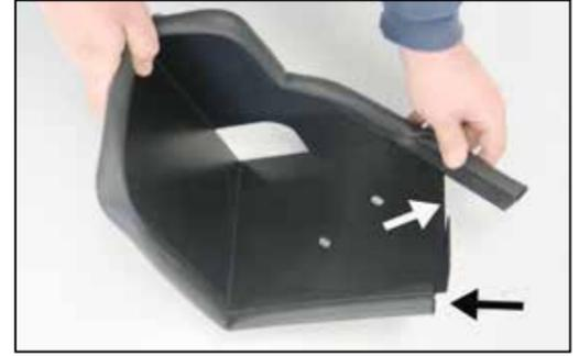
20. Install the provided edge trim onto the heat shield as shown.
