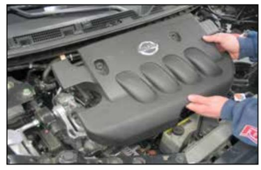
3. Remove the two bolts which secure the engine cover then remove the engine cover as shown.
