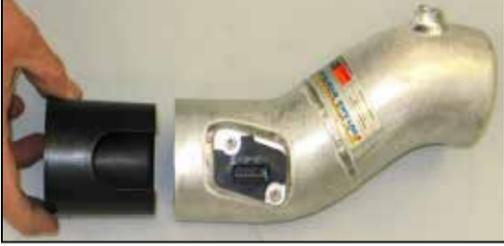
26. Install the mass air sensor venturi into the K&N® intake tube as shown.
