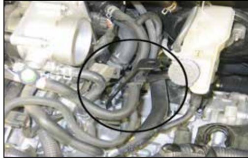
14. Unhook the evap/fuel lines from the mounting bracket, install the provided tube mounting bracket (083124) onto the water neck boss and secure with the provided hardware. Secure the evap/fuel lines to the hole provided in the tube mounting bracket.
