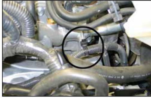
13. Unhook the wiring harness shown from the water neck housing location shown.
