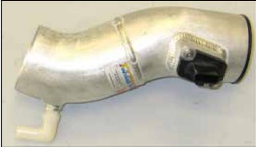
27. Install the provided 90° vent fitting onto the K&N® intake tube as shown.
