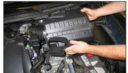
7. Loosen the hose clamp that secures the intake tube to the air box. Remove the stock air box from the vehicle.
