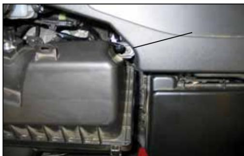
6. Remove the air box retaining bolt shown. **Note: This bolt is located at the rear of the air box near the strut tower.**
