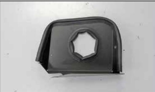
12. Install the provided edge trim onto the heat shield and into the hole of the edge rim as shown. **NOTE: Some trimming of the edge trim will be necessary.**
