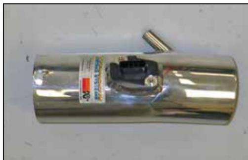
19. Install the mass air sensor into the K&N® intake tube and secure with the provided hardware.
