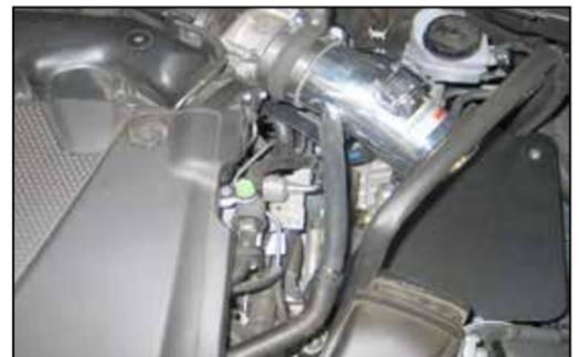
23. Install the crank case vent hose into the factory crank case vent hose and then connect the open end onto the K&N® intake tube as shown.
