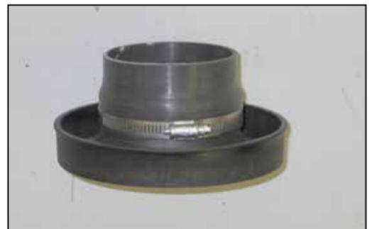
24. Install the silicone hose (084091) onto the air filter adapter and secure with the provided hose clamp as shown.
