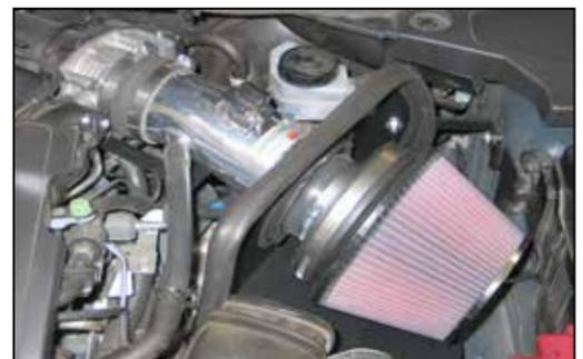
26. Install the K&N® air filter assembly onto the intake tube and secure with the provided hose clamp.
