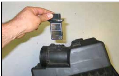
18. Remove the two screws securing the mass air sensor, and then remove the mass air sensor from the stock air box as shown.
