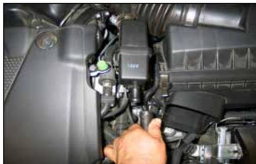
4. Release the crank case vent hose spring clamp and then disconnect the crank case vent hose from the intake tube resonator chamber.
