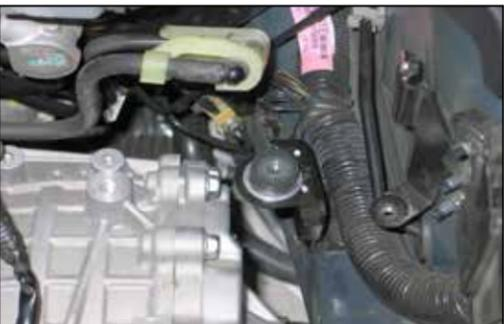
14. Install the shorter rubber mounted stud onto the rear air box mounting bracket as shown. **Note: Be sure to place a large fender washer on each side of the mounting bracket.**
