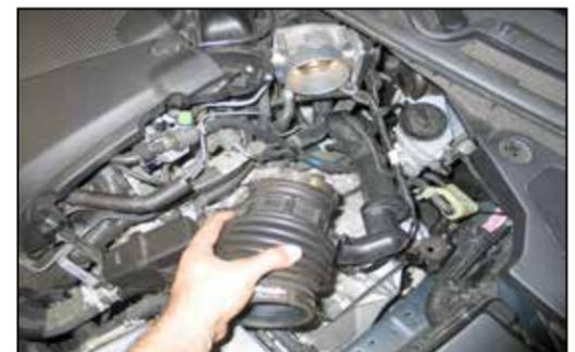
9. Remove the Stock Intake tube and intake tube resonator chambers as shown. **Note: Pull the lower intake tube resonator chamber firmly to release it from the mounting grommet.**
