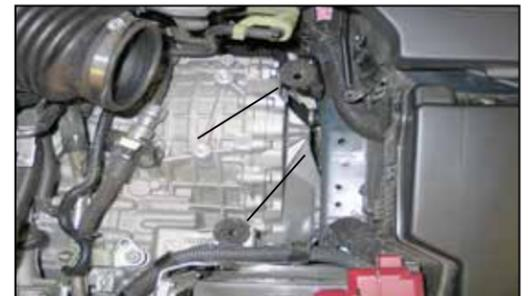
8. Remove the two air filter housing mounting grommets shown.
