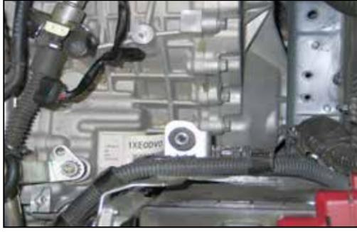
15. Install the longer rubber mounted stud onto the front air box mounting bracket as shown.
