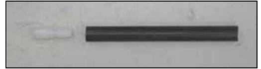
22. Install the hose mender into the crank case vent hose provided.
