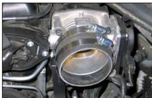
20. Install the silicone hose (08690) onto the throttle body and secure with the provided hose clamp.
