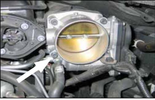
10. Remove the lower front throttle body mounting bolt shown. This bolt will be re-used in the next step.
