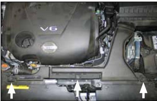
2. Remove the three bolts that secure the fresh air intake duct shown. These bolts will be re-used in a later step.
