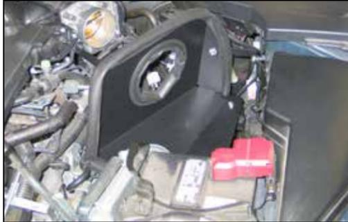
16. Install the heat shield assembly onto the rubber mounted studs installed in the previous steps and secure with the provided hardware. Secure the heat shield mounting bracket to the air box mounting bracket on the strut tower using the provided hardware.
