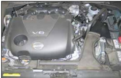
17. Re-install the fresh air intake duct onto the core support and into the heat shield and secure with the factory bolts.
