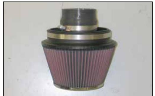
25. Install the K&N® air filter onto the air filter adapter assembly as shown.
