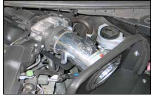
21. Install the K&N® intake tube into the silicone hose installed onto the throttle body and align it with the tube mounting bracket. Secure the intake tube with the hardware and hose clamp provided.
