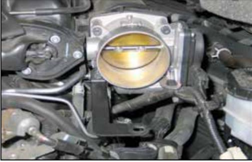
11. Using the bolt removed from the previous step, install the provided tube mounting bracket (070113) onto the throttle body as shown.
