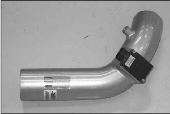
21. Install the mass air sensor into the intake tube and secure with provided hardware.
