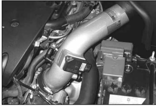
24. Install the K&N® intake tube into the silicone hose at throttle body and align with the mounting bracket installed in step #18. Secure the intake tube with the provided hose clamp and hardware. **NOTE: It may be necessary to reposition the positive battery cable to obtain proper clearance of the tube.**
