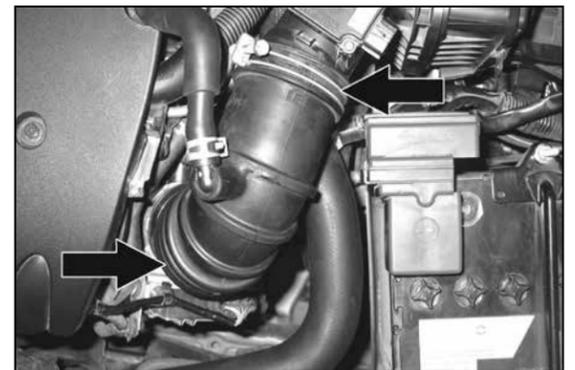
6. Loosen the two hose clamps that secure the stock intake tube to the throttle body and air filter housing.
