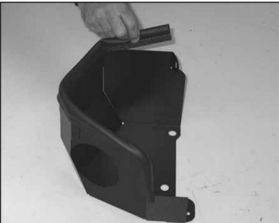
11. Install the long piece of the edge trim onto the heat shield as shown.
