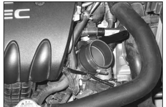
19. Install the provided silicone hose (08284) onto the throttle body and secure with the provided hose clamps.
