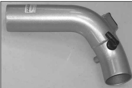
23. Install the 90° barbed fitting into the grommet that was installed into the K&N® intake tube in the previous step.
