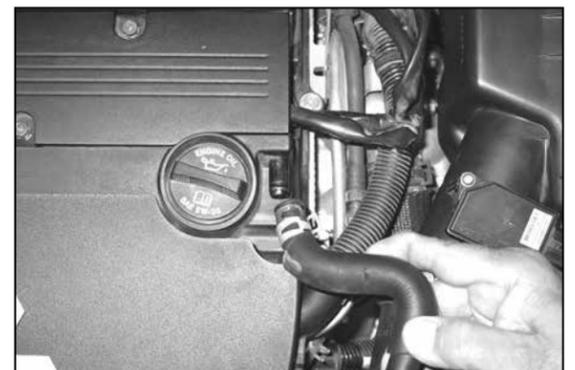
5. Release the spring clamp that secures the crank case vent hose to the valve cover port. Disconnect the crank case vent hose from the valve cover.
