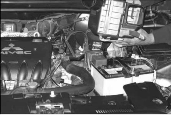
9. Lift up the air box assembly to unhook it from the mounting grommets and then remove the air box from the vehicle as shown.
