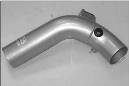
22. Install the provided 1/2" ID grommet (08064) into the intake tube as shown.
