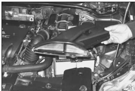
3. Remove the fresh air intake scoop from the vehicle.
