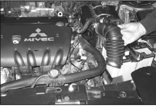
7. Remove the stock intake tube from the vehicle as shown.
