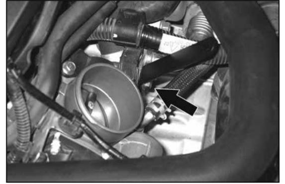
18. On vehicles equipped with an EGR tube, unhook the engine wiring harness from the clip and move the wiring harness rearward as shown. Install the intake tube mounting bracket (06724) onto the intake manifold and secure with the provided hardware.
