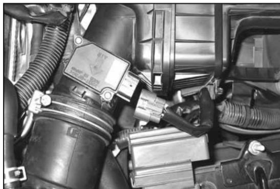
4. Disconnect the mass air sensor electrical connection and unhook the mass air sensor wiring harness from the air box.
