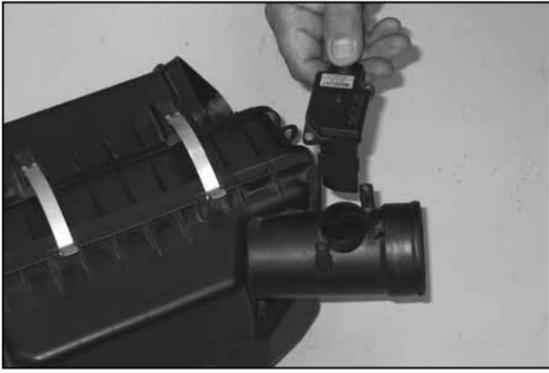
20. Remove the two screws that secure the mass air sensor into the factory air box and remove the mass air sensor as shown.
