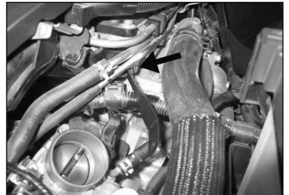
18b. Secure the provided tube mounting bracket (083140) to the engine using the provided hardware.
