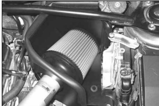
26. Install the K&N® air filter onto the intake tube and secure with the provided hose clamp.
