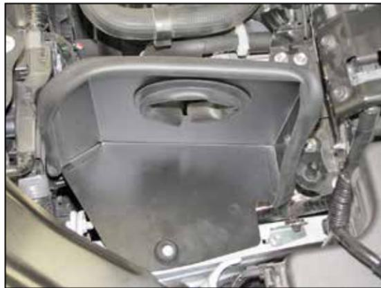
14. Install the heat shield onto the mounting stud and secure to the mounting bracket with the hardware provided.
