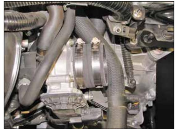
19. Install the provided coupling hose (08440) onto the throttle body and secure with the provided hose clamp.
