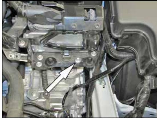
12. Remove the bolt shown from the battery tray.
