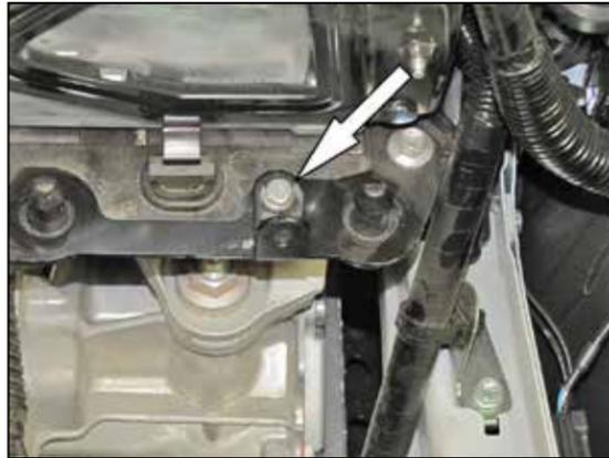
13. Install the heat shield mounting bracket (064313) onto the battery tray using the provided hardware.
