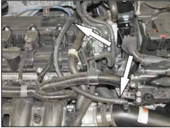
22. Install the provided crank case vent hose onto the valve cover port and then onto the 90° fitting in the intake tube.
