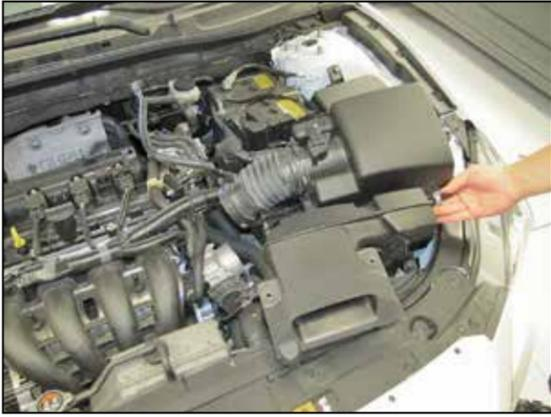
7. Lift up and remove the complete air box assembly from the vehicle.
