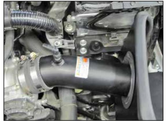
20. Install the K&N® intake tube assembly through the hole in the heat shield and then into the hose at the throttle body. Adjust the tube for best fit and secure with the provided hose clamp.
