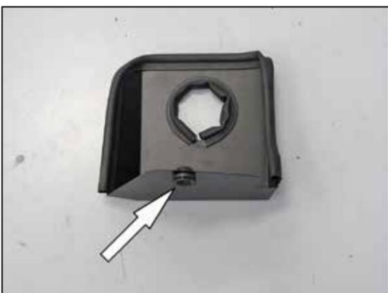
11. Install the mounting grommet from step 10 into the K&N® heat shield as shown.
