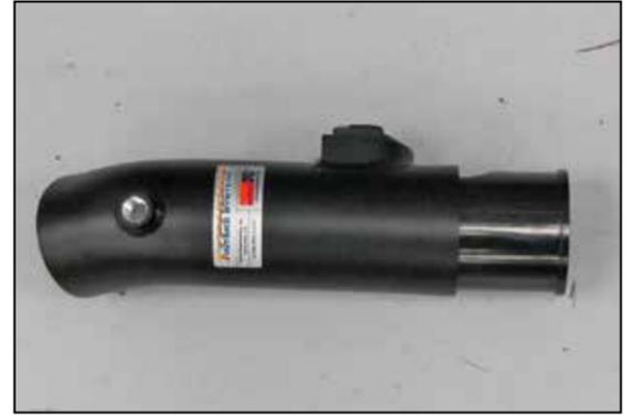
17. Apply several drops of the provided glue to the lip of the inner sleeve and then install the sleeve into the K&N® intake tube as shown.
