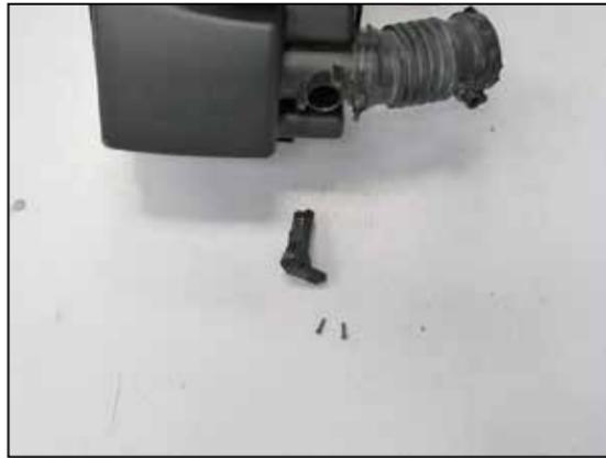
15. Remove the two screws securing the mass air sensor into the factory air box and then remove the mass air sensor.
