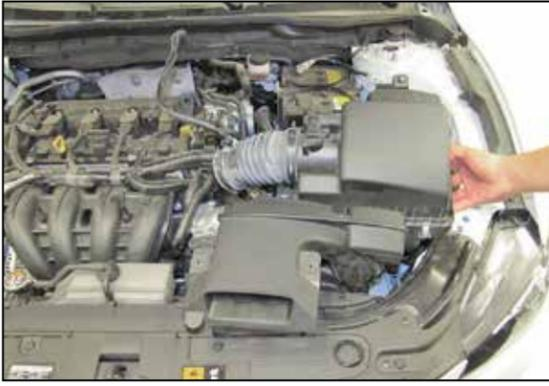
7. Disconnect the intake tube from the throttle body and then lift up the complete intake assembly and remove it from the vehicle.
