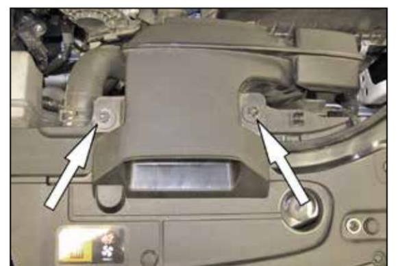
5. Remove the two bolts securing the fresh air inlet duct to the core support.
