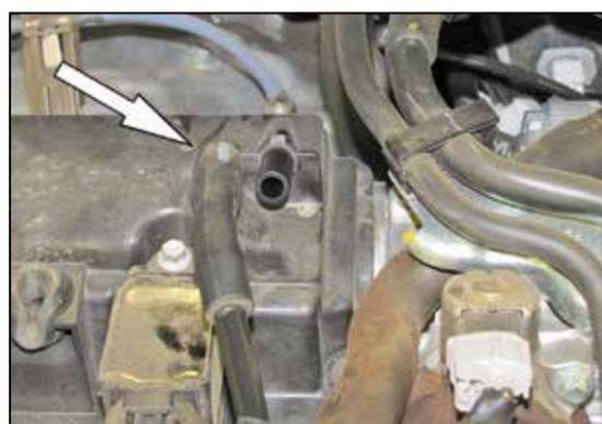
4. Disconnect the crank case vent tube from the valve cover port.
