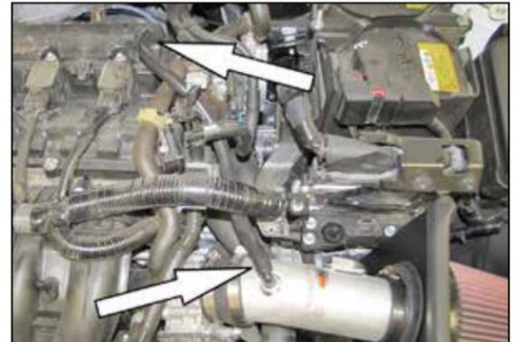
20. Install the provided crank case vent hose onto the valve cover port and then onto the fitting installed into the K&N® intake tube.
