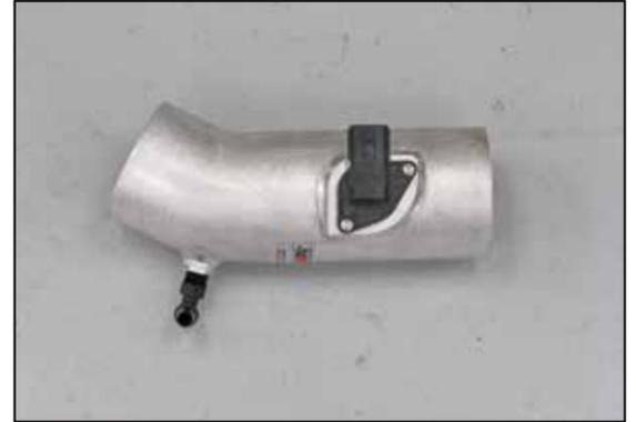
18. Install the mass air sensor into the K&N® intake tube and secure with the provided hardware.
