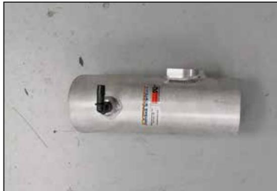
16. Install the provided 90° vent fitting into the K&N® intake tube as shown. **NOTE: Plastic NPT fittings are easy to cross thread. Install the vent fitting "hand" tight, then turn it two complete turns with a wrench.**
