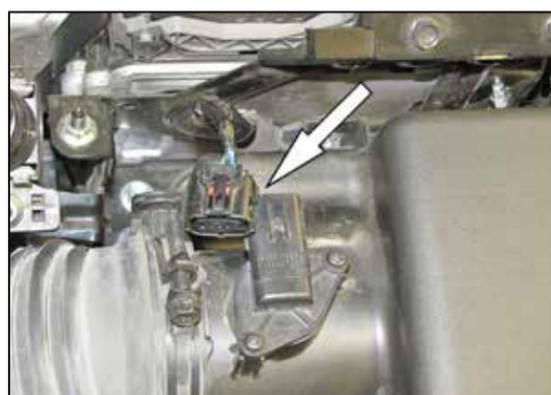
3. Disconnect the mass air sensor electrical connection and unhook the wiring harness from the air box.
