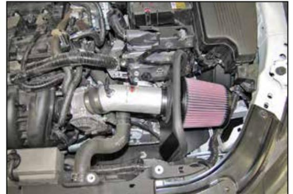
19. Install the K&N® Air filter through the heat shield, install the intake tube into the air filter and then into the coupling hose. Adjust the tube and filter for best fit and then secure with the provided hose clamps.
