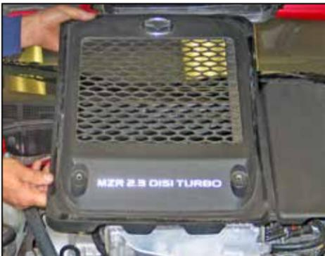
2. Remove the two bolts that secure the intercooler cover, then remove the intercooler cover as shown.
