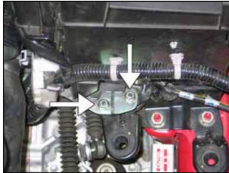
14. Remove the two nuts that secure the wiring harness loom as shown.
