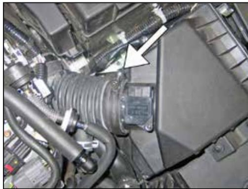
4. Loosen the hose clamp that secures the intake tube to the upper airbox housing.
