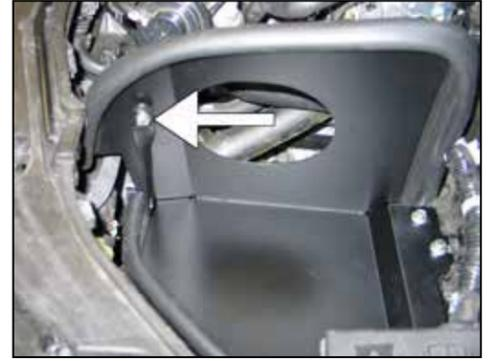
17. Install the heat shield mounting bracket (07945) onto the heat shield with the provided hardware.
