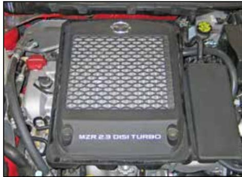
29. Reinstall the engine cover and secure with the factory bolts (removed in step #2).
