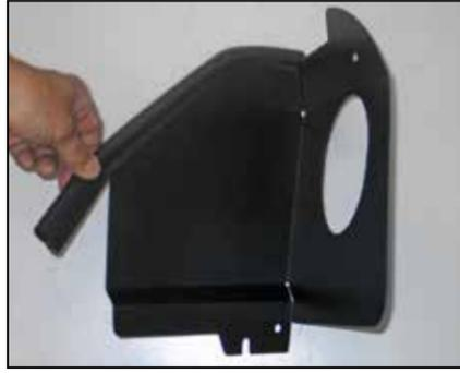
12. Install the short edge trim onto the heat shield as shown.
