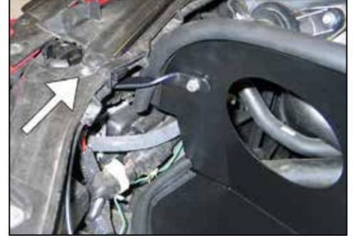
18. Swing the heat shield bracket up under the core support, then mount to the core support using the provided hardware as shown.
