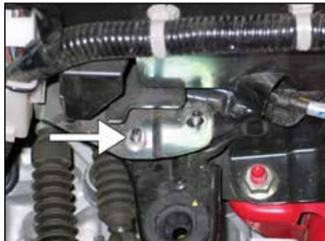
15. Install the provided spacer onto the inner wiring loom stud as shown.
