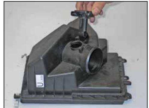
19. Remove the mass air sensor from the stock upper airbox housing as shown.
