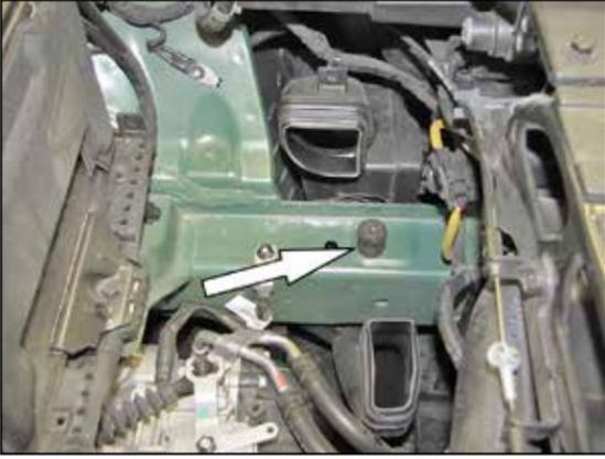
8. Install the 1" male to female rubber mounted stud onto the frame rail as shown.
