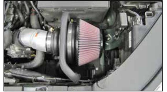
18. Install the K&N® air filter onto the filter adapter and secure with the provided hose clamp.
