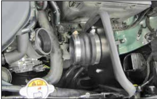
15. Install the provided hump hose (5-576) onto the filter adapter and secure with the provided hose clamp.
