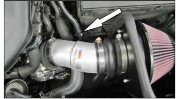
19. Install the crank case vent hose onto the 90° fitting and secure with the factory spring clamp.
