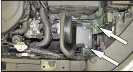
13. Install the heat shield assembly onto the rubber mounted stud and align the mounting bracket with the mounting hole. Secure the heat shield with the provided hardware.
