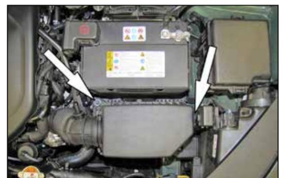
6. Remove the two bolts securing the air box.
