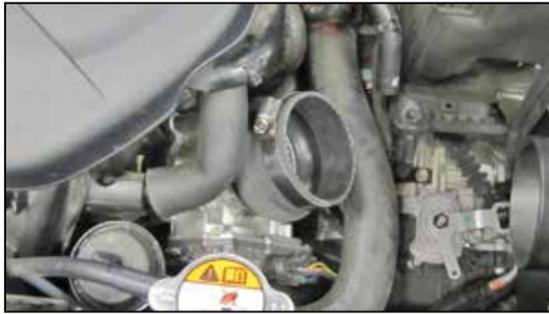
14. Install the provided hump hose (08421) onto the throttle body and secure with the provided hose clamp.
