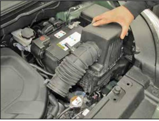
7. Lift up and remove the air box and intake tube from the vehicle.
