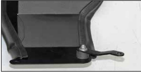
12. Install the mounting bracket (26545) onto the rubber mounted as shown using the provided hardware.
