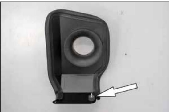
11. Install the 6mm male to male rubber mounted stud onto the heat shield as shown using the provided hardware.
