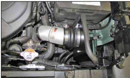
17. Flex the heat shield assembly towards the driver's side fender and then install the K&N® intake tube into the coupling hoses. Adjust the tube and heat shield for best fit and then secure with the provided hose clamps.
