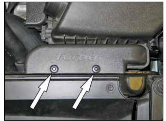
5. Push the centers of the retaining pins down to release the fresh air intake scoop.
