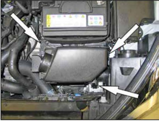
7. Remove the three bolts securing the air filter housing assembly and then lift up and remove the air filter housing assembly from the vehicle.
