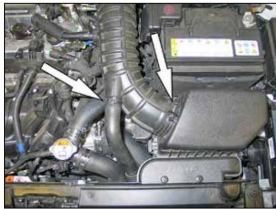
3. Loosen the hose clamp securing the intake hose to the air box and release the spring clamp securing the air injection hose and then disconnect the air injection hose.
