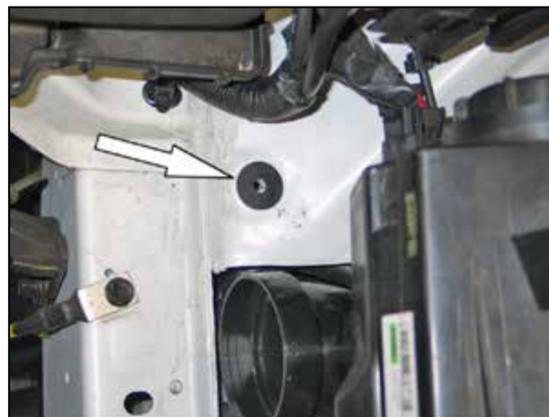
15. Set the provided rubber fender washer onto the air box mounting location on the inner fender as shown.
