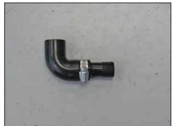
21. Install the provided hose mender into the 90° air injection hose and secure with the provided hose clamp.
