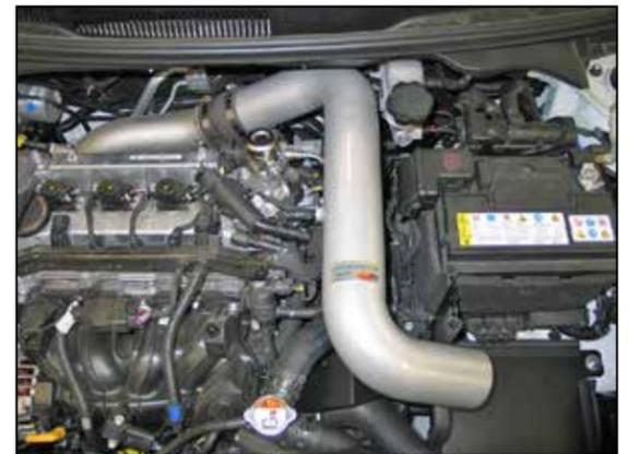
19. Install the K&N® intake tube into the silicone hose and align with the mounting bracket. Secure the tube with the hose clamp and hardware provided.
