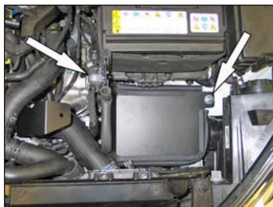
16. Install the heat shield assembly and secure it the two air box mounting locations with the provided hardware as shown.
