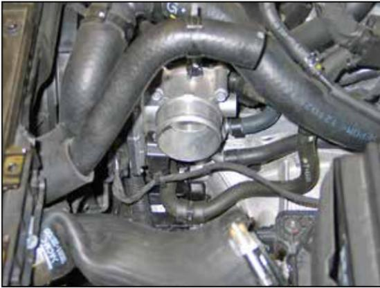
8. Remove the small cover that is installed onto the hose clamp screw securing the intercooler charge hose, then loosen the hose clamp and disconnect the charge hose from the throttle body inlet.
