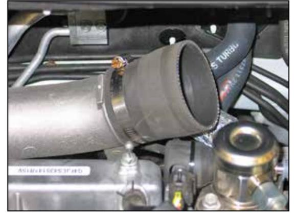
17. Install the provided silicone hose (08096) onto the turbo inlet as shown and secure with the provided hose clamp.
