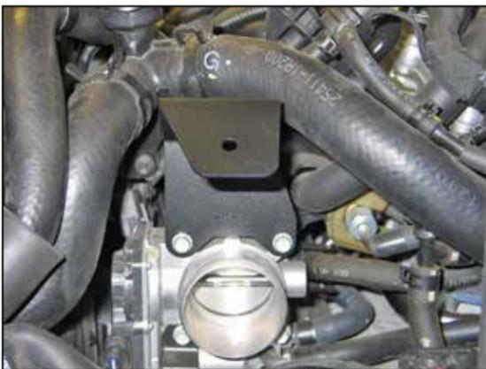
10. Install the provided tube mounting bracket (064303) onto the throttle body and secure with the factory bolts from the previous step.
