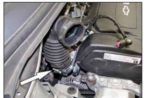
5. Loosen the hose clamp securing the intake hose to the throttle body and then remove the intake tube from the engine.
