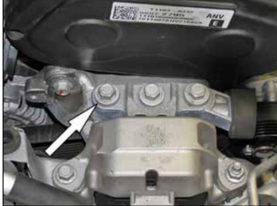
13. Remove the rear engine mounting bolt shown.
