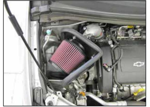
17. Install the K&N® air filter onto the intake tube and secure with the provided hose clamp.
