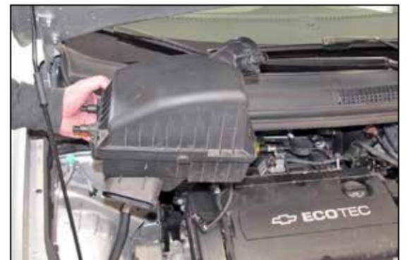
4. Lift up and remove the air box from the vehicle as shown.
