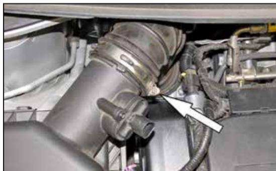
3. Loosen the hose clamp securing the intake hose to the air box and then disconnect the intake hose from the air box.
