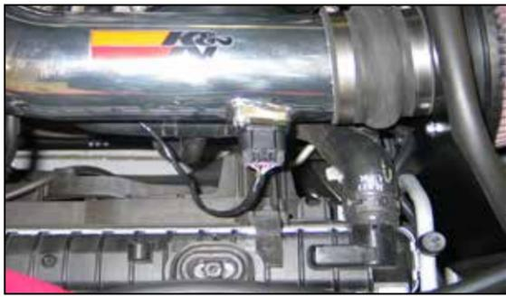
24. Reconnect the mass air sensor electrical connection.
