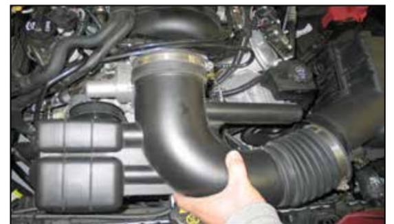
6. Remove the stock intake tube as shown.
