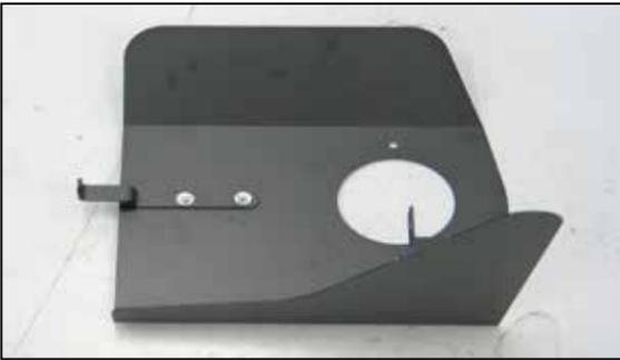
11. Install the heat shield mounting bracket (083126) onto the heat shield as shown using the provided hardware.
