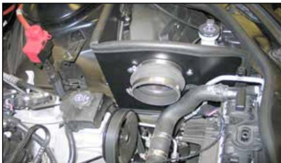
17. Install the silicone hose (08418) onto the filter adapter and secure with the provided hose clamp.
