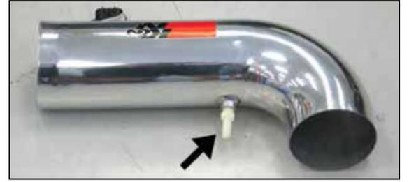
20. Install the provided 1/4npt fitting into the K&N® intake tube as shown.
