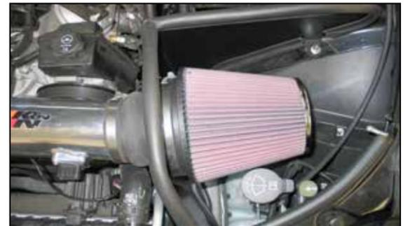
23. Install the K&N® air filter onto the filter adapter and secure with the provided hose clamp.
