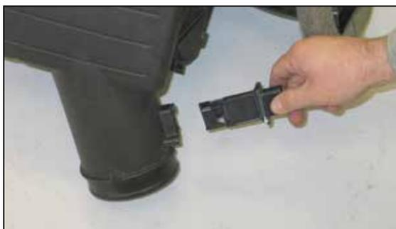
18. Remove the two screws and then remove the mass air sensor from the factory air box.
