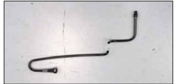
22a. On 2014 and later vehicles, it will be necessary to cut the crank case vent tube as shown. Then connect the cut section of tube to the oil filler cap. Attach the supplied hose to the to the trimmed section of crank case vent tube,
