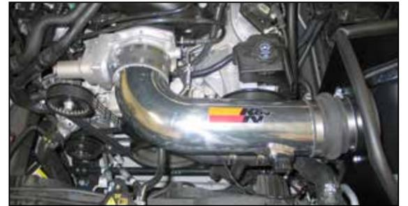
21. Install the K&N® intake tube assembly into the silicone hose at the filter adapter and then into the silicone hose at the throttle body and secure with the provided hose clamps.
