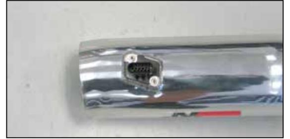
19. Install the mass air sensor into the K&N® intake tube and secure with the provided hardware.
