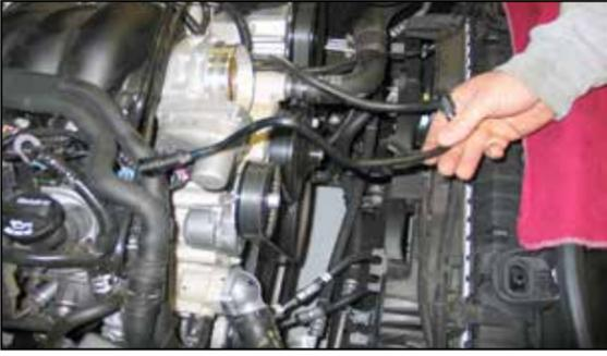
7. Rotate the crank case vent tube 180°, then release the retainer at the valve cover port and the remove the crank case vent tube.
