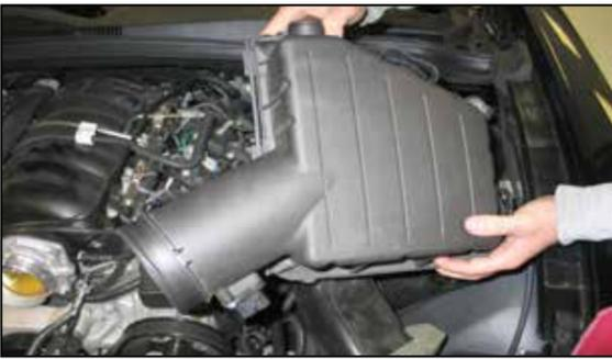
9. Lift up and remove the air box from the vehicle.
