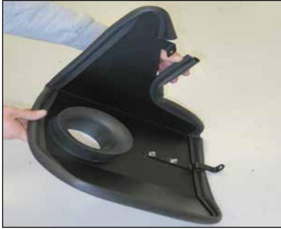
13. Install the edge trim onto the heat shield as shown.
