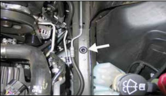
10. Remove the air box mounting grommet shown from the frame rail.
