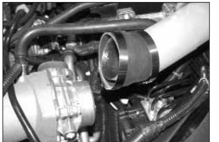
17. Install the silicone hose and provided hose clamps onto the K&N intake tube as shown.
