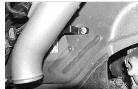
20. From underneath the vehicle, secure the K&N intake tube to the mounting bracket installed in step #15.
