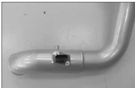
13. Install the mass air sensor onto the K&N intake tube and secure with the provided hardware.
