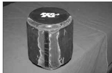
23. Install the K&N Drycharger on the the K&N air filter.
