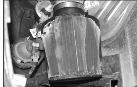
24. Install the K&N air filter onto the intake tube and secure it with the provided hose clamp as shown.
