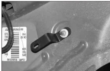
15. Install the provided "Z" bracket (010033) onto the factory air box mounting stud and secure with the factory nut as shown.
