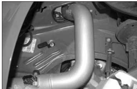
16. From underneath the vehicle, slide the K&N intake tube up and through the hole in the fender well.
