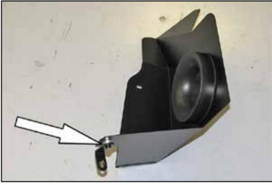
7. Install the provided heat shield bracket (064326) onto the heat shield and secure with the provided hardware.
