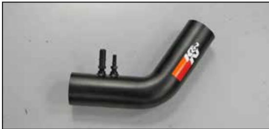
13. Install the provided quick disconnect fittings into the K&N® intake tube as shown.
