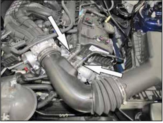
2. Release the locking tabs and disconnect the crank case vent hose and EVAP vent hose from the factory intake tube.
