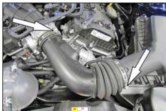
3. Loosen the hose clamps securing the factory intake tube to the throttle body and air filter housing then remove the intake tube from the vehicle.
