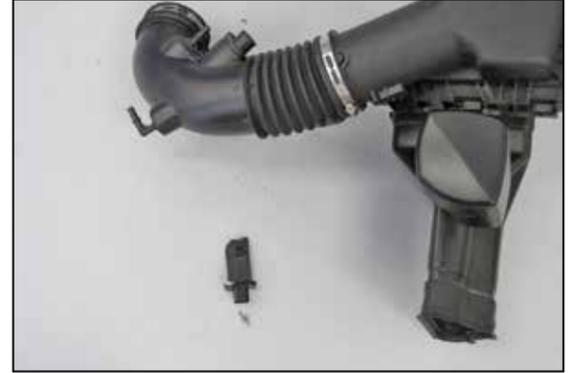
18. Remove the mass air sensor from the factory air filter housing.
