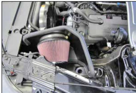
15. Install the K&N® air filter onto the adapter and secure with the provided hose clamp, then secure the heat shield and brackets to the air filter housing mounting location using the provided hardware.
