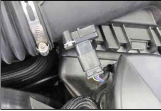
7. Release the locking tab and then disconnect the mass air sensor electrical connection.
