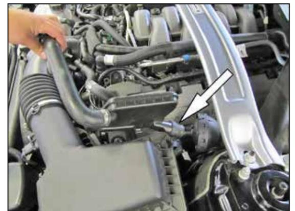
5. Cut the clamp that secures the sound tube/ chamber to the sound drum and then disconnect the sound tube/chamber from the sound drum.
