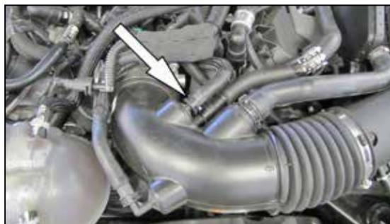
3. Depress the locking tab and then disconnect the idle bypass hose from the intake tube.
