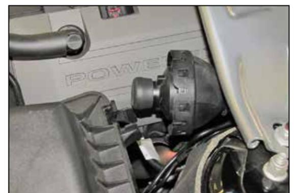
6. Install the provided cap onto the sound drum.
