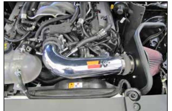
20. Install the K&N® intake tube into the hose at the filter adapter and then into the hose at the throttle body, adjust the tube and hoses for best fit and then secure with the provided hose clamps.
