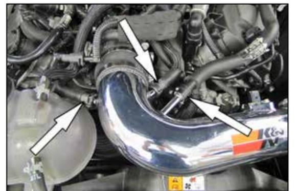
21. Connect the crank case vent, EVAP vent and idle by pass lines to the quick disconnect fittings installed into the K&N® intake tube.
