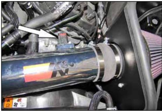
22. Connect the provided mass air sensor extension harness into the factory mass air sensor connection and then connect the other end to the mass air sensor.
