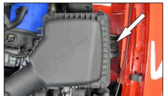
5. Remove the bolt securing air box to the inner fender.
