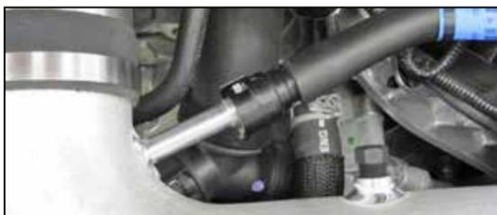
19. Connect the crank case vent hose to the quick connect fitting on the K&N® intake tube.
