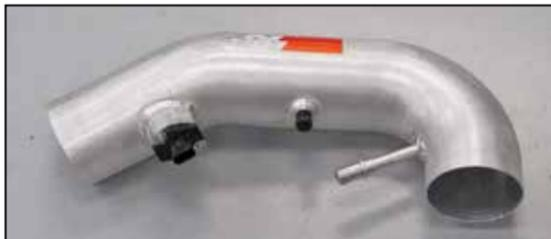
15. Install the mass air sensor into the K&N® intake tube and secure with the hardware provided.
