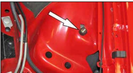
11. Install the provided rubber mounted stud onto the inner fender at the factory air box mounting location.
