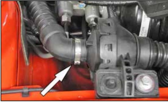
7. Cut the clamp securing the engine sound tube to the drum and then remove the engine sound tube from the vehicle. Install the provided cap plug onto the drum.
