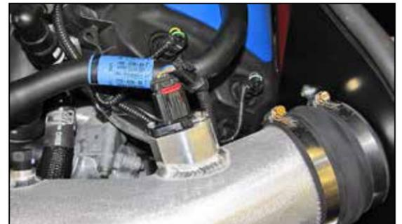
21. Reconnect the mass air sensor electrical connection.
