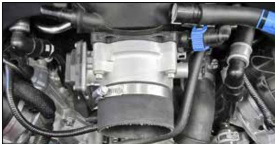
16. Install the provided coupling hose (08698) onto the throttle body and secure with the provided hose clamp.
