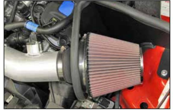
20. Install the K&N® air filter onto the filter adapter and secure with the provided hose clamp.
