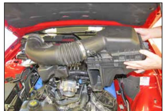
6. Disconnect the intake tube from the throttle body then remove the complete intake system from the vehicle.
