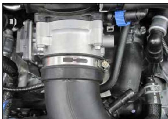
4. Loosen the hose clamp securing the intake tube to the throttle body.
