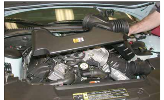
7. Remove the stock intake tube assembly from the vehicle.
