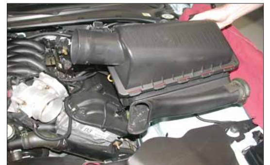
9. Pull up firmly on the air box to dislodge it from the retaining pin, and then remove the air box from the vehicle.
