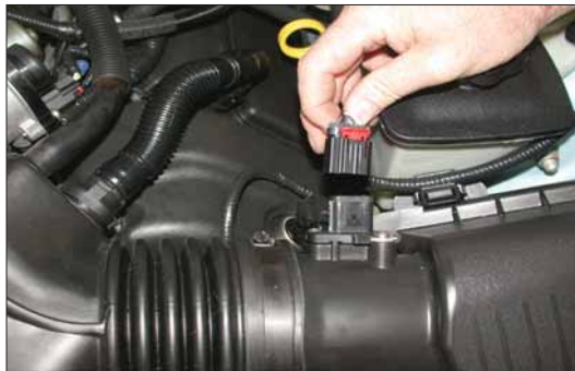
4. Pull back the red locking tab on the mass air sensor electrical connection, and then disconnect the mass air sensor electrical connection.
