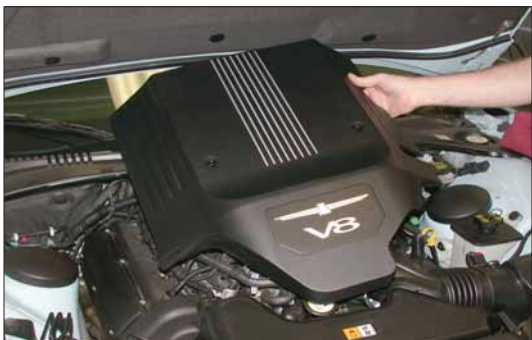
3. Pull up on the rear of the engine cover to dislodge from the retaining mounts, and then remove the engine cover from the engine.
