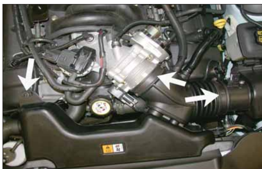
6. Loosen the hose clamps at the throttle body and the factory air box, and then remove the intake tube retaining nut shown.
