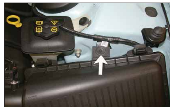
8. Remove the air box retaining bolt shown.
