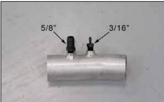
14. Install the 3/16" vent fitting and 5/8" vent fitting into the K&N intake tube as shown.
