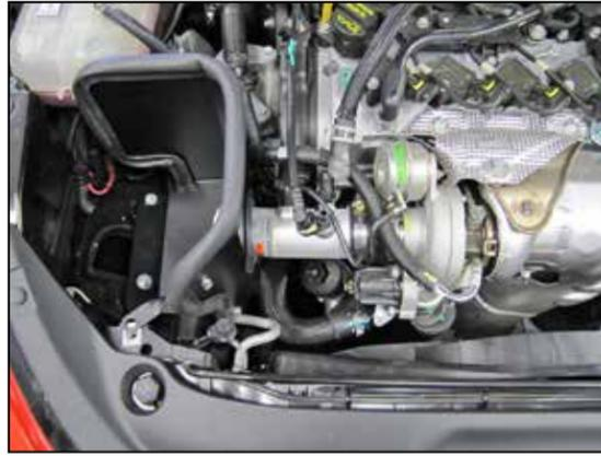
15. Tilt the heat shield towards the fender, install the K&N intake tube through the hole in the heat shield and then install into the silicone hose on the turbo. Rotate the tube so the vent fittings align with the factory hoses and then secure the tube with the provided hose clamp.
