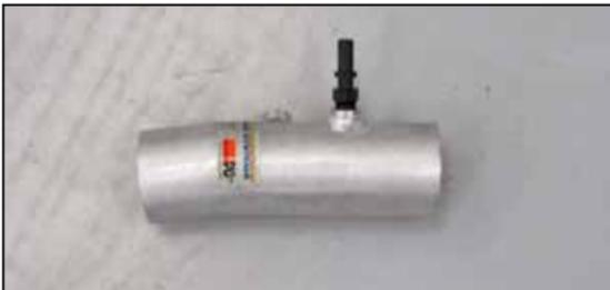
13. Install the provided quick disconnect fitting into the K&N intake tube as shown.
