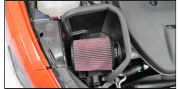
20. Install the K&N air filter and secure with the provided hose clamp.
