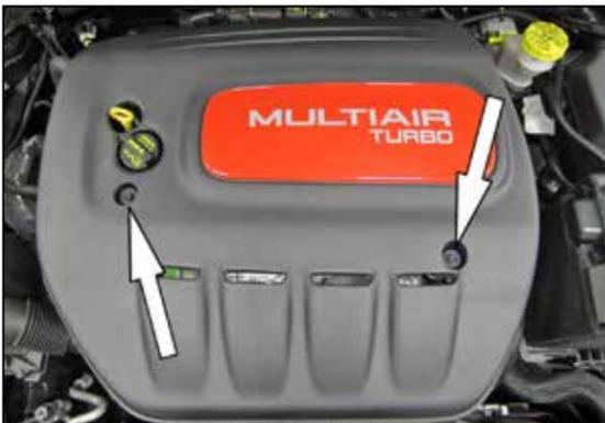
2. Remove the two bolts securing the engine cover and then remove the cover from the vehicle.
