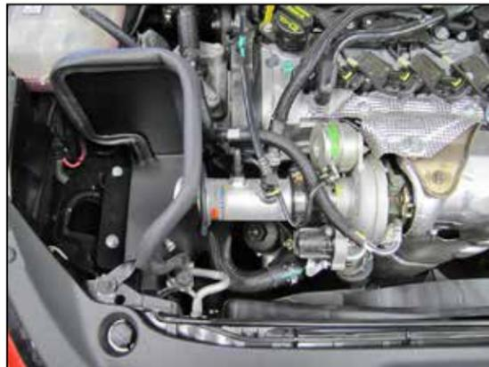
17. Connect the crank case vent hose, EVAP vent hose and BOV hose the fittings installed into the K&N intake tube.
