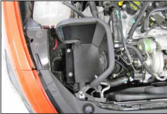
11. Install the heat shield into position so the stand-offs set into the air box mounting grommets.
