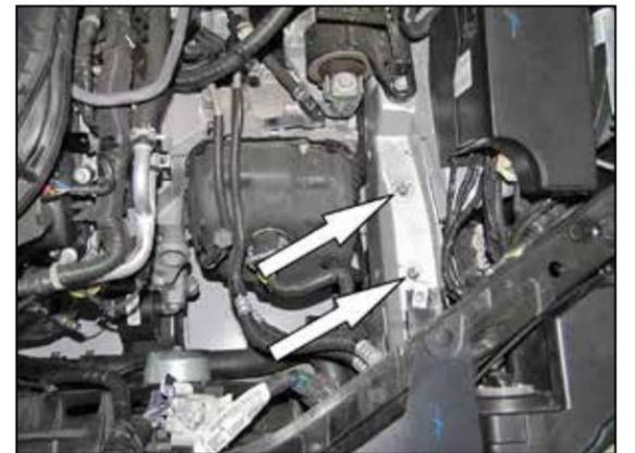
7. Remove the two air box mounting studs shown.
