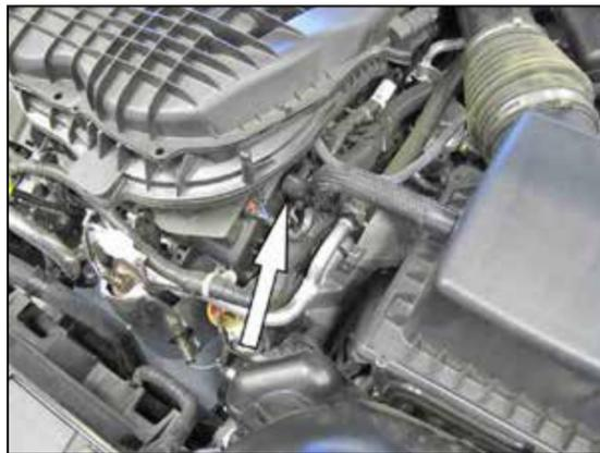
4. Disconnect the crank vent hose from the valve cover.
