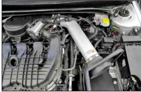
15. Install the K&N® intake tube into the silicone hose at the filter adapter and then into the hose at the intake plenum, then secure with the provided hose clamp.
