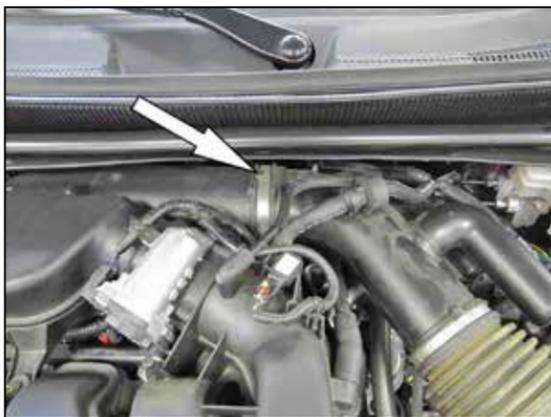
3. Loosen the hose clamp securing the intake hose to the intake plenum.
