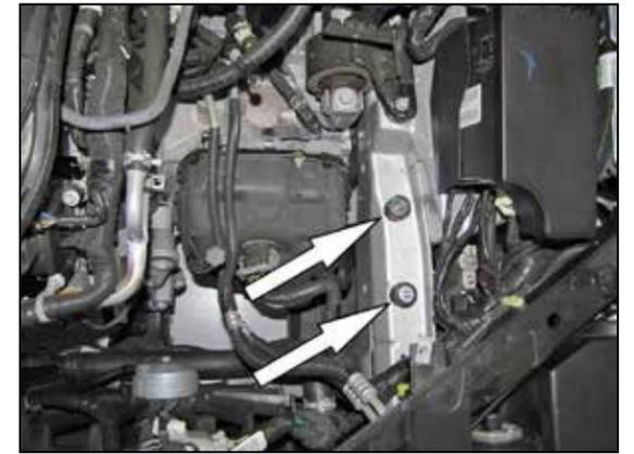
8. Install the two provided rubber mounted studs into the air box mounting stud locations.
