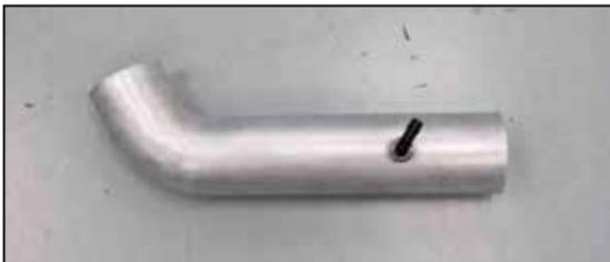
14. Install the 90° vent fitting into the intake tube as shown.
