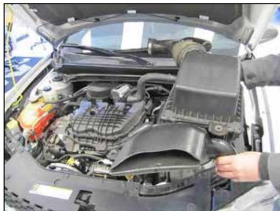
6. Lift up the complete stock intake system and remove it from the engine compartment.
