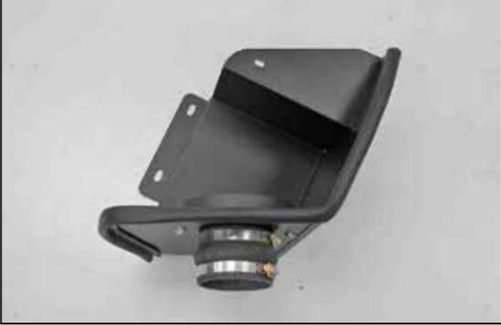
11. Install the provided silicone hose (08699) onto the filter adapter and secure with the provided hose clamp.
