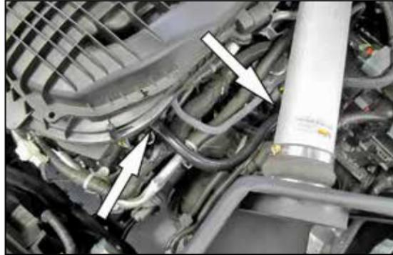
16. Install the provided crank case vent hose onto the fitting installed into the K&N® intake tube and then onto the factory fitting on the valve cover.
