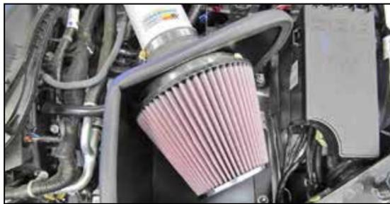
17. Install the K&N® air filter onto the filter adapter and secure with the provided hose clamp.
