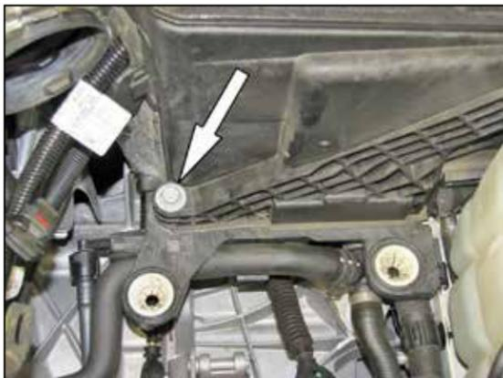
11. Remove the battery cover bolt shown.
