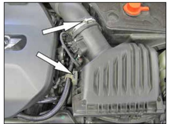
5. Loosen the hose clamp securing the intake tube to the air filter housing and unhook the ground cable from the air filter housing, then lift up the air filter housing and remove it from vehicle.
