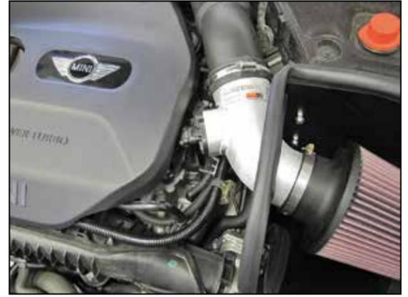
17. Reconnect the mass air sensor electrical connection.
