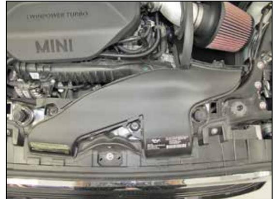
18. Reinstall the fresh air intake scoop and secure with the factory hardware.
