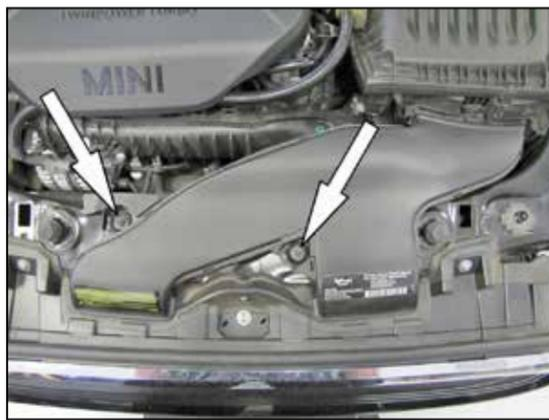
3. Remove the two nuts that secure the fresh air intake scoop and then remove the scoop from the vehicle.
