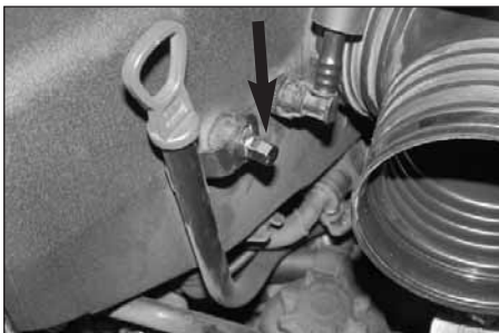
27. Remove the cap nut from the dipstick tube as shown.
