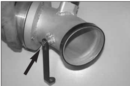
25. Install the provided bracket onto the K&N intake tube assembly using the provided hardware as shown.
