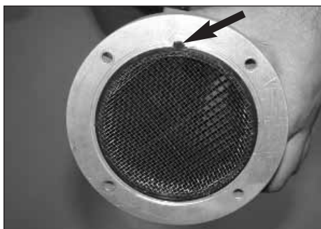
21. Install the stock mass air straightener from step 19 into the K&N intake tube as shown.
