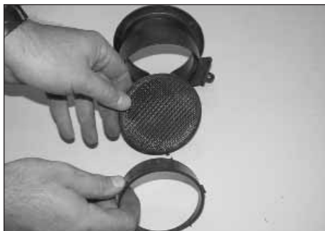
19. Disassemble the velocity stack as shown.
