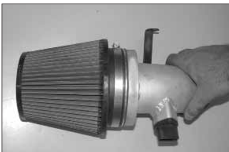
26. Install the K&N Air Filter onto the K&N intake tube assembly and secure with the provided hose clamp as shown.
