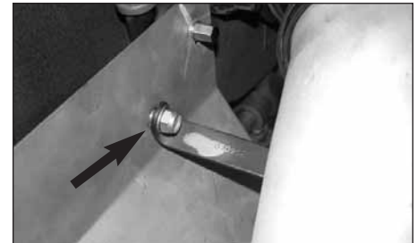
32. Line up the bracket with the hole on the heat shield and secure with the provided hardware as shown.
