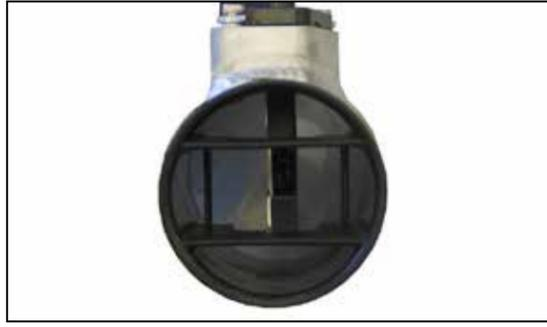
15a. Install the provided venturi into the end of the intake tube as shown.
