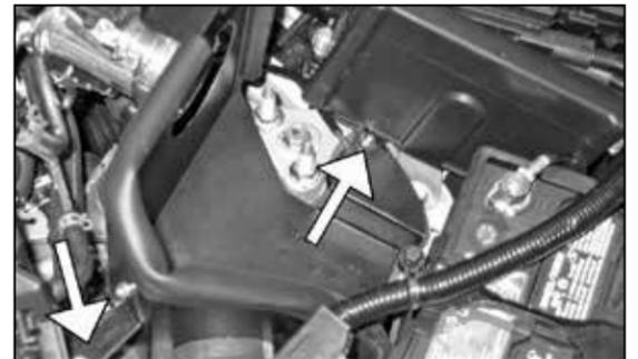
25. Attach the "L" bracket to the heat shield, and then install a bolt through the the hole on the ECU bracket to the threaded boss on the heat shield. Then attach the factory air inlet hose to the heat shield.
