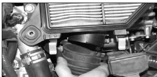
7. Remove the air inlet hose from the lower factory airbox.
