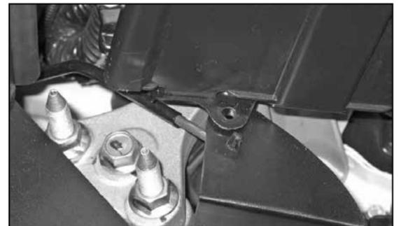
24. Install clip to the hydraulic line then attach to hole in heat shield.
