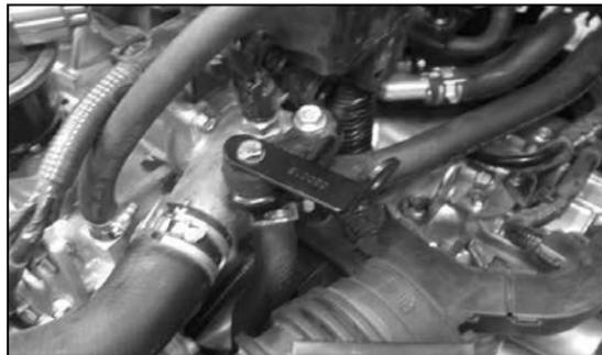
19. Install the "L" bracket onto the rubber mounted stud as shown.
