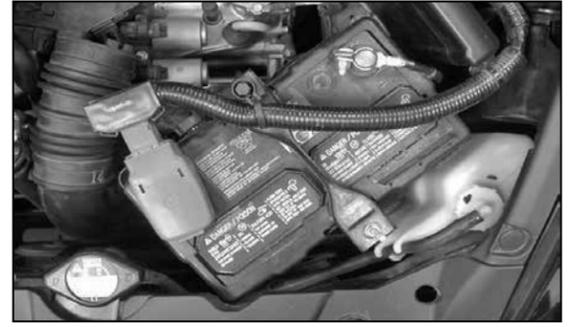
21. Loosen the positive battery cable and unclip the battery wire harness, adjust battery cable as shown. Then resecure the battery.
