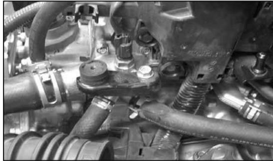
18. Secure the rubber mounted stud onto the other factory airbox mounting point.
