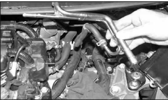
11. Using pliers, remove the coolant hose from the thermostat housing and the throttle body adaptor (a small amount of coolant may drain, have a cup ready to catch the fluid).
