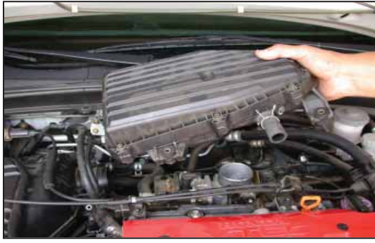
10. Pull firmly upwards to remove the throttle body plenum as shown.
