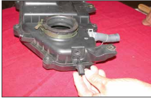
16. Remove the air temperature sensor from the throttle body plenum as shown.
