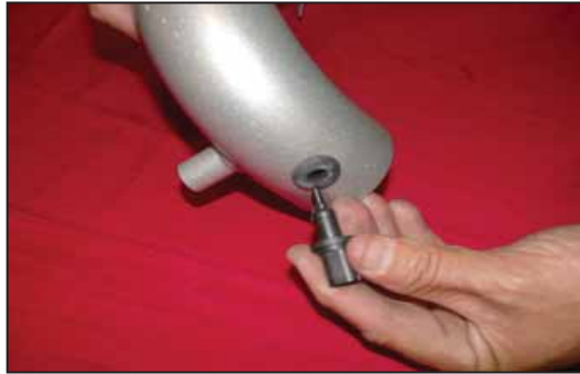
17. Install the provided rubber grommet into the hole on the K&N® intake tube, then install the air temperature sensor into the grommet as shown. NOTE: Before installing the grommet and air temperature sensor, inspect the inside of the tube for any debris, then clean the inside out with water and a towel. Inspect the tube one more time before proceeding to the next step.
