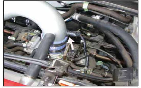
21. Reconnect the air temperature sensor electrical connection as shown.
