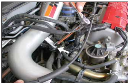
19. Secure the bracket to the rubber mounted stud using the provided hardware, but do not tighten completely at this time.
