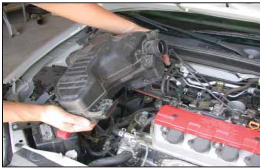
12. Unclip the throttle cable and cruise control cable (if equipped), then, remove the resonator by pulling upwards as shown. NOTE: K&N Engineering, Inc., recommends that customers do not discard factory air intake.
