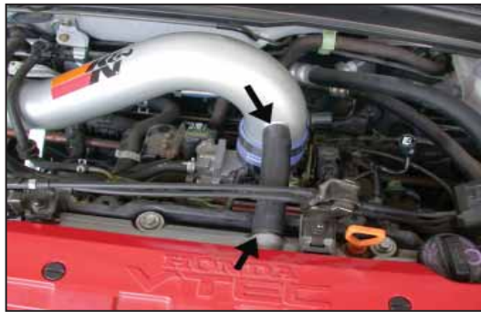
20. Install the provided silicone hose onto the crankcase vent on the cam cover, then connect the other end to the vent on the K&N® intake tube as shown.
