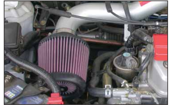
22. Install the K&N® air filter onto the K&N® intake tube and secure with the provided hose clamp. Adjust for best fit and clearance then tighten all hardware.
