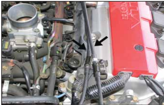
13. Secure the throttle cable and cruise control cable (if equipped) to the stock clips as shown.
