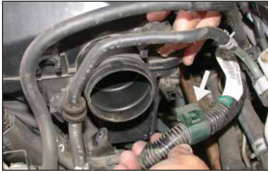
11. Using a flat blade screwdriver, unclip the wire harness from the resonator as shown.
