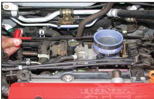
14. Install the silicone hose and hose clamps onto the throttle body. Do not tighten at this time.
