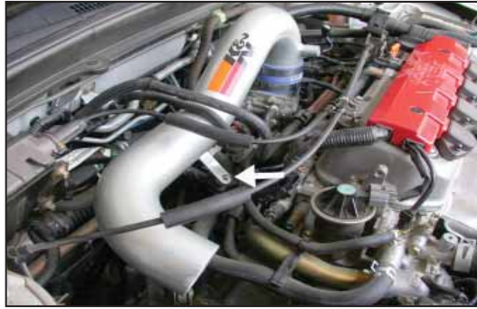
18. Install the K&N® intake tube onto the throttle body, then, line up the bracket with the rubber mounted stud as shown. Tighten hose clamps at this time.
