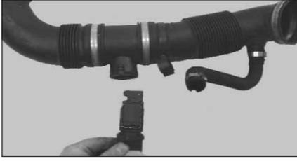
21. Unscrew and remove the MAS from the original intake pipe as shown.
