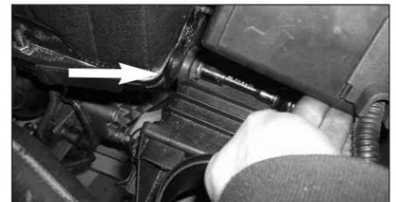
11. Undo the air box mounting nut located on the front of the battery tray as shown.
