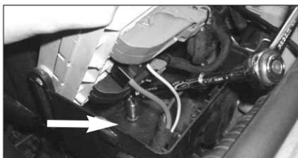
9. Carefully remove the black cover at the bottom of the box and undo the indicated nut.
