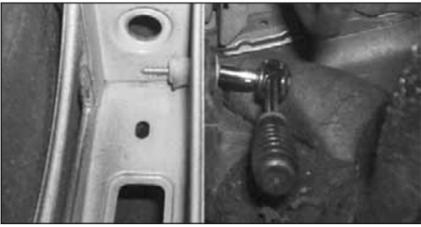
17. From underneath the car, remove the intake snorkel securing screw. Now carefully remove the intake snorkel from the vehicle by pulling it downwards.
