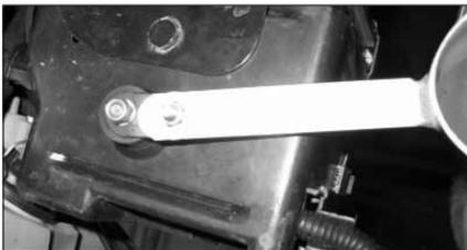
26. From underneath the car, fit the bracket onto the rubber stud. Align the tube for best clearance and fully tighten all its securing hardware.
