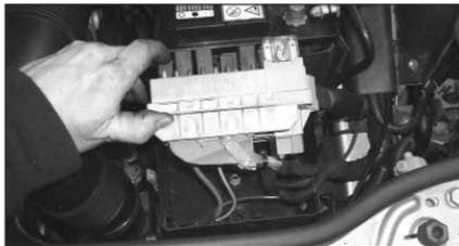
8. Open the fuse and relay box. Unclip the front of the fuse and relay tray and tilt it backwards as shown.
