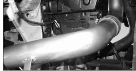
30. Fit the "B" tube into the silicone hump hose as shown, but don't tighten the #40 hose clamp yet!
