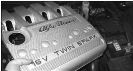
2. Remove the oil filler cap, undo the 4 fixing screws and remove the engine cover from the vehicle as shown.
