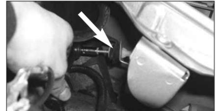
12. Undo the indicated intake snorkel securing screw from the left hand inner wing as shown.
