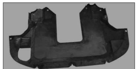
13. Taking all the necessary safety precautions, as per manufacturer's instructions raise the front of the vehicle and support it with axle stands. Then, remove the under tray from the vehicle.
