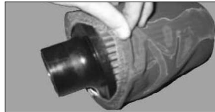
32. Fit the K&N Drycharger over the K&N Filter as shown. **NOTE:** The Drycharger's water repellent properties will last up to 2 years. See parts list to re-order Drycharger if necessary.
