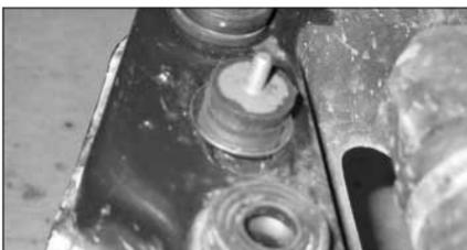
27. Place a large metal washer and the M/F rubber stud over the slot in the lower air box mounting plate as shown.
