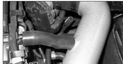
34. Fit the breather hose supplied between the intake tube and the cam cover as shown. Trim the hose as necessary.
