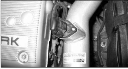
35. Re-install the engine cover and reconnect the MAS electrical connector as shown.
