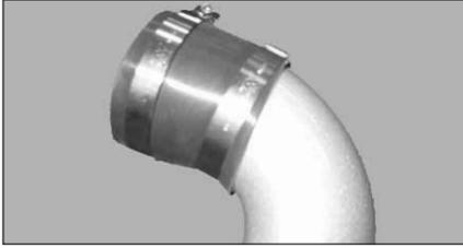
24. Fit the stepped silicone sleeve onto the intake tube using a #40 hose clamp supplied, and fit the #44 hose clamp over the sleeve as shown. Don't fully tighten either yet!
