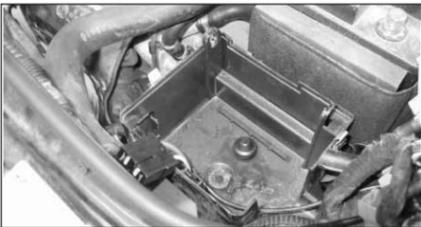
18. Re-install the mounting bracket and fuse and relay box, using their respective original nuts as shown.
