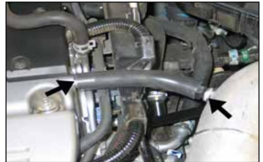
24. Install the provided crank case vent hose onto the valve cover vent port and fitting onto the K&N® intake tube.
