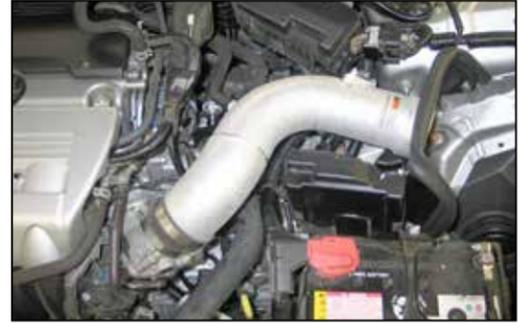
23. Install the K&N® intake tube through the heat shield, into the silicone hose at the throttle body and align with the tube mounting bracket previously installed. Align and then secure with the provided hose clamp and hardware.
