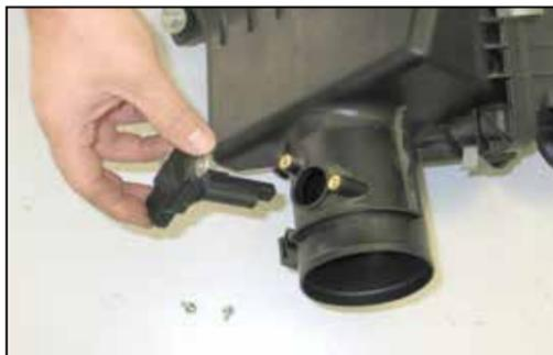
20. Remove the two screws that secure the mass air sensor to the air box then remove the mass air sensor from the air box.
