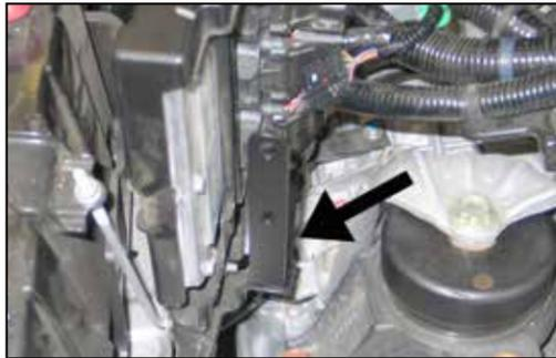
18. Install bracket number 083120 onto the ECM mounting bracket as shown.
