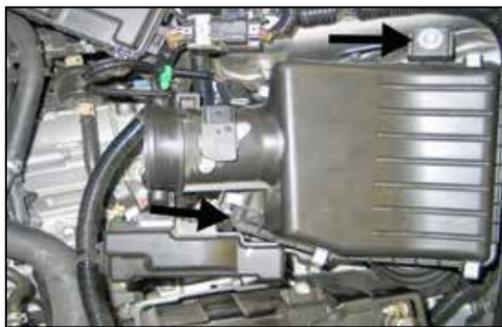
6. Loosen the two bolts securing the air box assembly to the inner fender and ECU bracket.
