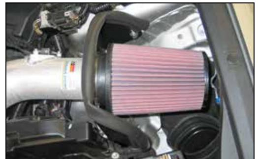
25. Install the K&N® filter and secure with provided hose clamp.
