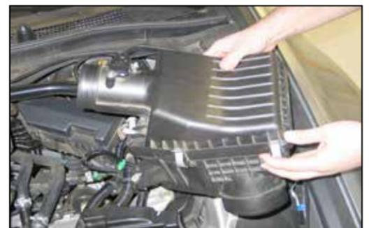
7. Remove the air filter assembly from the vehicle. **NOTE: K&N Engineering, Inc., recommends that customers do not discard factory air intake.**
