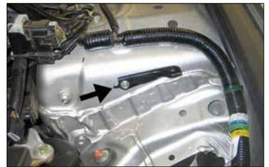
8. Remove the rear air filter mounting bracket shown from the strut tower.
