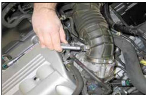
4. Release the spring clamp and disconnect the crank case vent tube from the intake tube.
