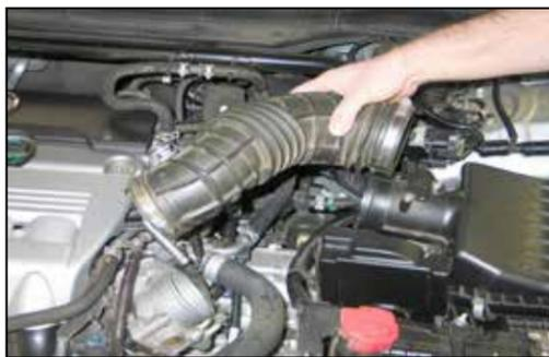
5. Remove the intake tube from the vehicle.
