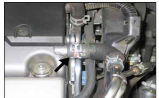
9. Release the spring clamp then unhook the crank case vent hose from the valve cover.
