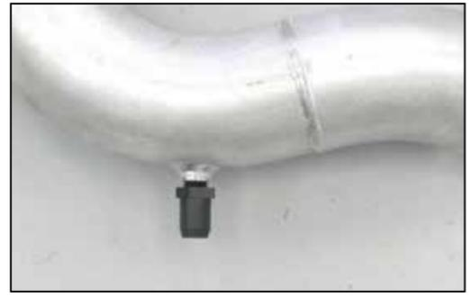
22. Install the provided NPT vent fitting into the intake tube as shown.
