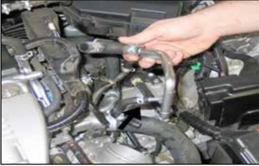
11. Release the spring clamp and then disconnect the steel by-pass hose assembly from the bypass hose attached to the thermostat housing.
