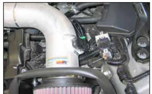
26. Reconnect the mass air sensor electrical connection.
