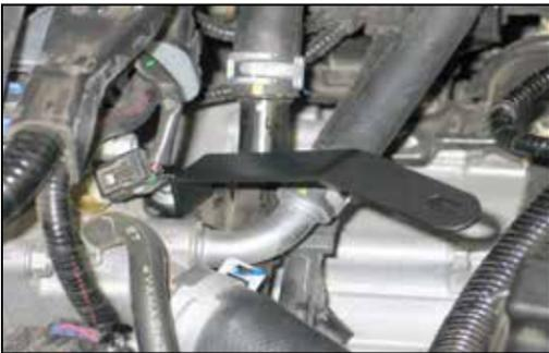
14. Secure bracket number 083121 to the thermostat housing as shown with the provided hardware.
