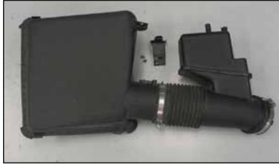
17. Remove the two screws securing the mass air sensor and then remove the mass air sensor from the upper air box housing.
