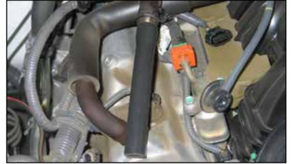
23. Install the crank case vent hose assembly into the factory crank case vent hose as shown.
