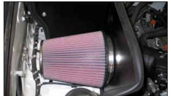
26. Install the K&N® air filter and secure with the provided hose clamp.
