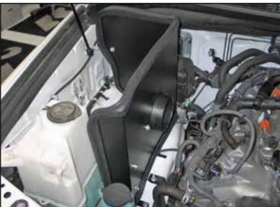
14. Set the heat shield into the engine compartment and secure the factory nuts and with the provided hardware.
