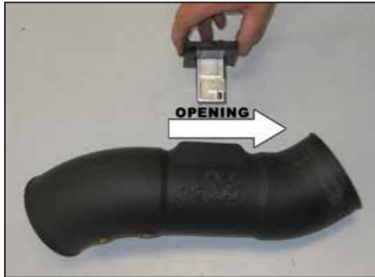
20. Install the mass air sensor assembly into the K&N® intake tube so that the opening in the sensor faces the filter end of the tube as shown.
