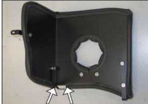
17. Install the provided longer edge trim onto the heat shield as shown.
