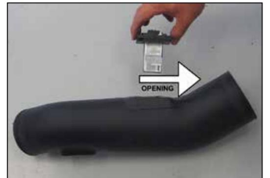
23. Install the mass air sensor assembly into the K&N® intake tube as shown using the provided hardware.
