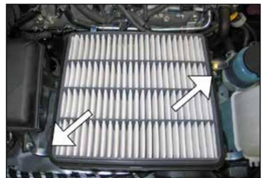
9. Loosen the two bolts securing the lower airbox into the vehicle.
