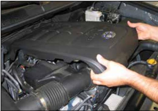
2. Lift up the engine cover to dislodge it from the mounting studs and then remove the engine cover from the vehicle.
