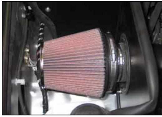
29. Install the filter assembly onto the K&N® intake tube and secure with the provided hose clamp. **NOTE: Drycharger® air filter wrap; part # RF-1042DK is available to purchase separately. To learn more about Drycharger® filter wraps or look up color availability please visit <http://www.knfilters.com>®.**
