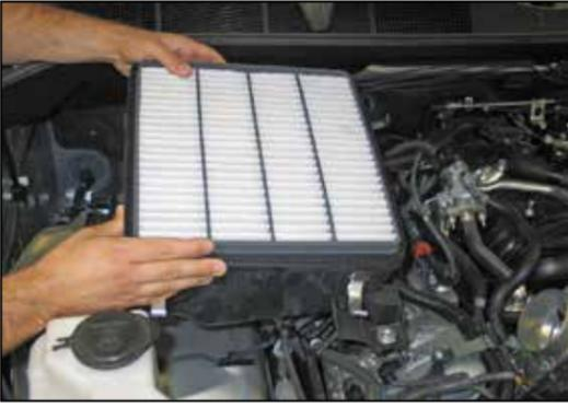
10. Remove the lower airbox from the vehicle.
