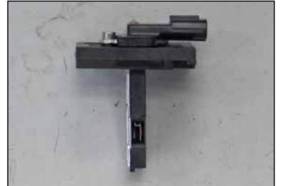
22. Install the mass air sensor into the K&N® mass air sensor adapter and secure with the provided hardware.
