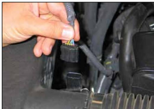
5. Disconnect the mass air sensor electrical connection and unhook the wiring harness from the upper airbox.
