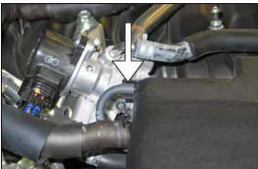
3. Disconnect the fuel pressure regulator vacuum hose from the intake tube.
