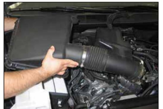
8. Remove the upper airbox/intake hose assembly from the vehicle.
