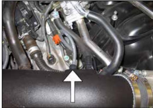
30. Connect the fuel pressure regulator vent line to the NPT fitting installed into the K&N® intake tube.
