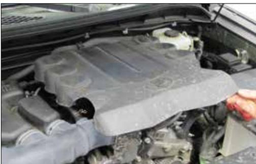
2. Lift up the engine cover to dislodge it from the mounting grommets and then remove the cover from the vehicle.
