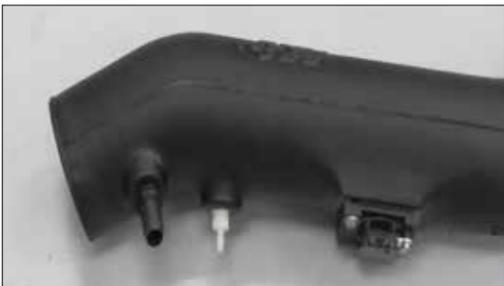
27. Install the 3/16 vent fitting into the K&N® intake tube as shown.
