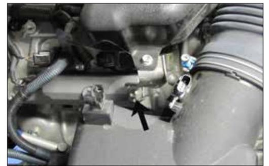
6. Remove the bolt which secures the tube mounting bracket to the engine valve cover.
