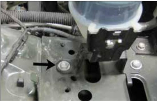
10. Remove the rear P/S reservoir mounting bolt shown.
