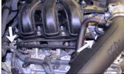
30. Connect the provided fuel pressure vent line to the fuel pressure regulator and then connect the open end to the 3/16 vent fitting in the K&N® intake tube.
