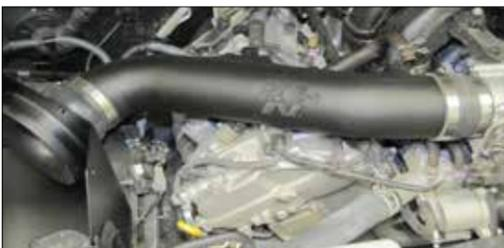
28. Install the K&N® intake tube into hump hose at the filter adapter and then into the silicone hose at the throttle body, align the tube for proper fit and then tighten the hose clamps.
