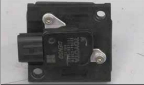
24. Install the mass air sensor into the K&N® mass air sensor adapter and secure with the provided hardware.
