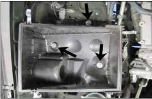
9. Loosen and remove the three bolts securing the lower air box and then remove the lower air box from the vehicle.
