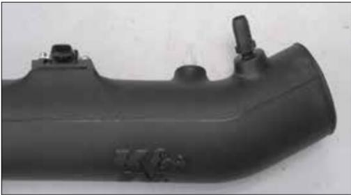
26. Install the 5/8 vent fitting into the K&N® intake tube as shown.
