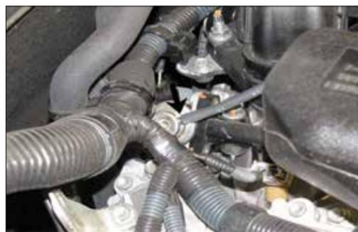
4. Unhook the fuel pressure vent line from the fuel pressure regulator.
