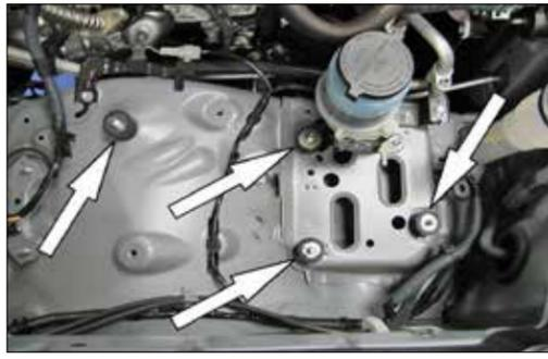
12. Install the four rubber mounted studs into the factory air box and P/S reservoir as shown.
