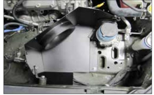
19. Set the heat shield onto the rubber mounted studs and the secure with the provided hardware.
