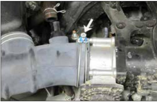
7. Loosen the hose clamp which secures the intake tube to the throttle body.
