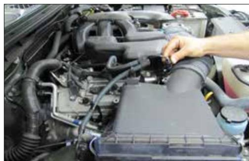
3. Disconnect the mass air sensor electrical connection and then unhook the wiring harness from the air box.
