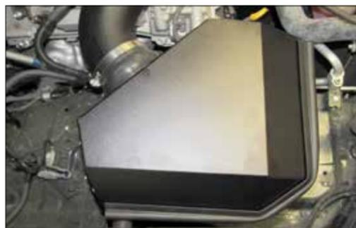
33. Install the heat shield cover onto the heat shield and secure with the provided hardware.
