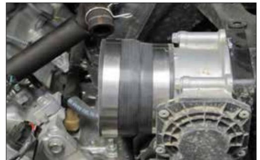
21. Install the provided silicone step hose (084091) onto the throttle body and secure with the provided hose clamp.
