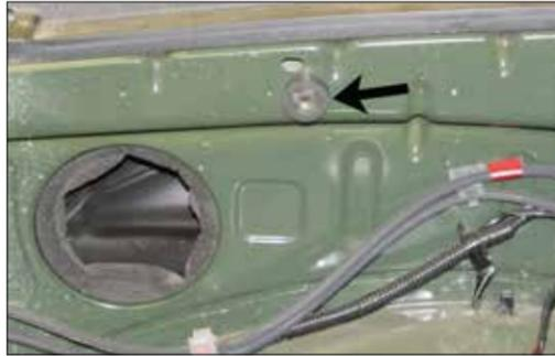
13. Install the 6mm rubber mounted stud into the inner fender location shown.
