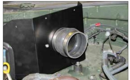
20. Install the provided silicone hump hose (084057) onto the filter adapter and secure with the provided hose clamp.
