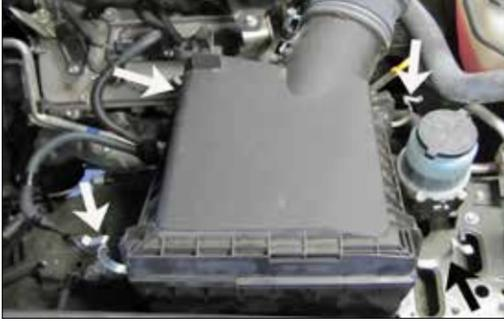
8. Release the four clips which secure the upper air box to the lower air box and then remove the intake tube and upper air box from the vehicle.
