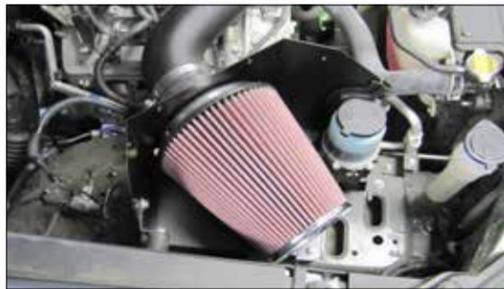
31. Install the K&N® air filter onto the filter adapter and secure with the provided hose clamp.
