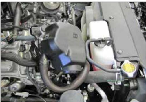
11a. Lift up the air injection pump, disconnect the electrical connection and then set the air injection pump over to side.
