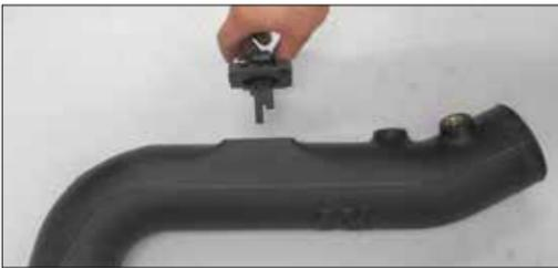
25. Install the mass air sensor assembly into the K&N® intake tube and secure with the provided hardware.
