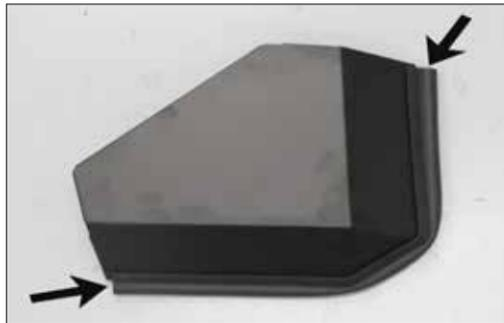
32. Install the remaining 19" piece of edge trim onto the heat shield cover as shown.
