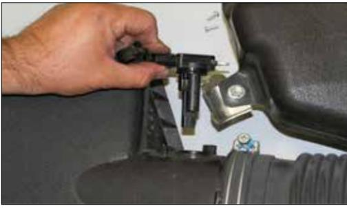
23. Remove the screws which secure the mass air sensor to the factory air box and then remove the mass air sensor from the air box.
