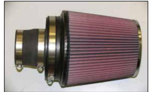
26. Install the silicone hose (08698) onto the air filter as shown and secure with the provided hose clamp.
