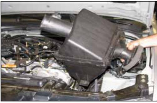
10. Pull firmly on the air box to dislodge it from the mounting grommets and remove it from the vehicle.
