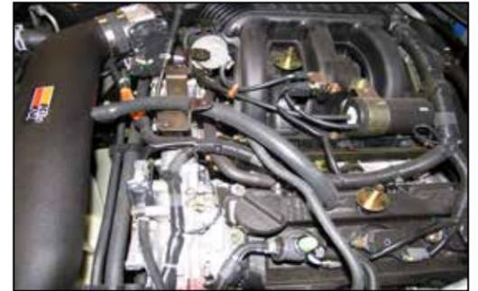
24. Attach the provided crank case vent hose to the valve cover and K&N® intake tube as shown and secure with the provided hose clamps.
