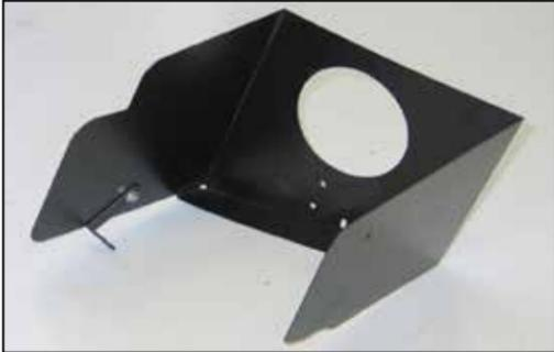
12. Install "L" Bracket (070632) onto the heat shield with the provided hardware.
