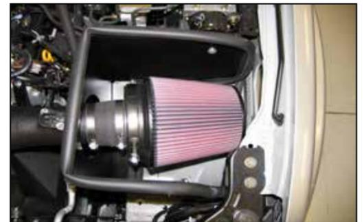
27. Install the air filter assembly onto the intake and secure with the provided hose clamp.
