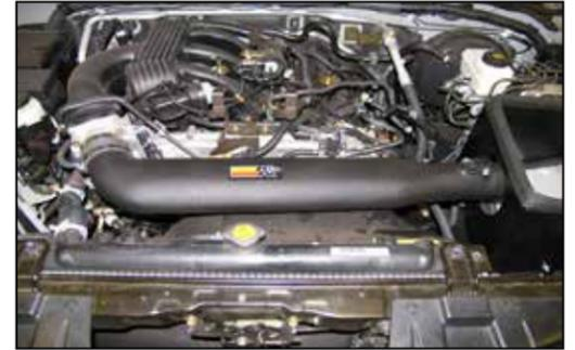
23. Install the K&N® intake tube into the silicone hose at the throttle body and align with the tube mounting bracket installed in step #16. Secure with the provided hardware and hose clamp.
