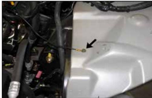
18. Remove the bolt, which secures the ground strap to the inner fender.
