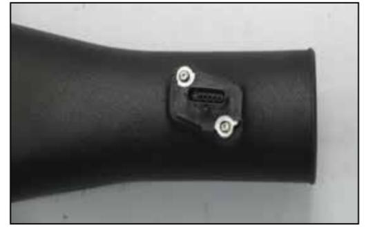
22. Install the mass air sensor into the K&N® intake tube and secure with the screws removed in step #21 and the provided spacers.
