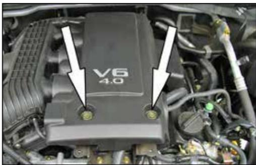
28. Reinstall the engine cover removed in step #4 and secure with the factory mounting bolts.
