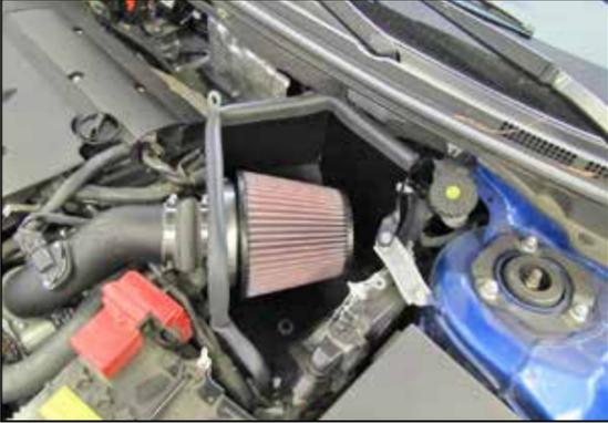
23. Install the K&N® air filter and secure with the provided hose clamp.
