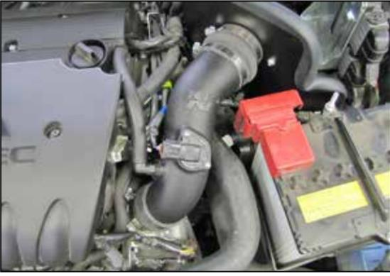
22. Connect the mass air sensor electrical connection.
