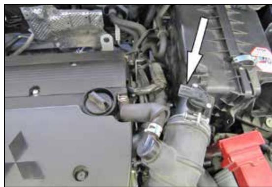
3. Disconnect the mass air sensor electrical connection and unhook the harness from the air filter housing.
