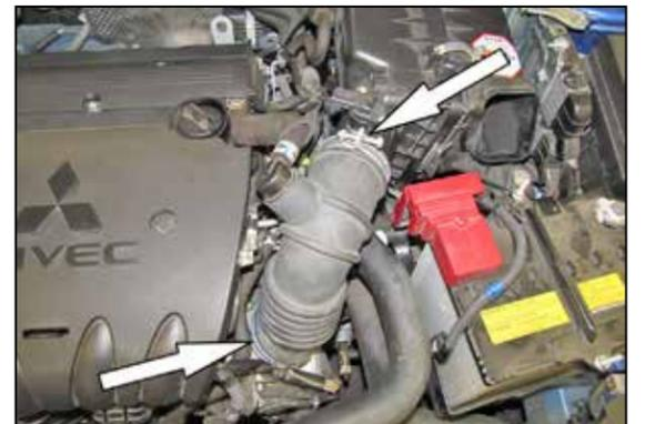
5. Loosen the hose clamps securing the factory intake tube to the air filter housing and throttle body and then remove the intake tube from the vehicle.
