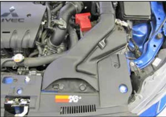
24. Reinstall the fresh air intake scoop and secure with the factory fasteners.
