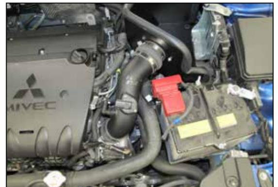
20. Install the K&N® intake tube into the coupler on the filter adapter and then into the coupler on the throttle body. Adjust the tube for best fit and then secure with the provided hose clamps.
