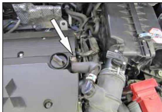
4. Release the spring clamp securing the crank case vent hose to the valve cover and then disconnect the hose from the valve cover.
