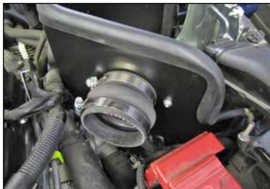
15. Install the provided coupling hose (087121) onto the filter adapter and secure with the provided hose clamp.
