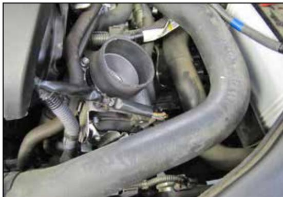
14. Install the provided coupling hose (08440) onto the throttle body and secure with the provided hose clamp.
