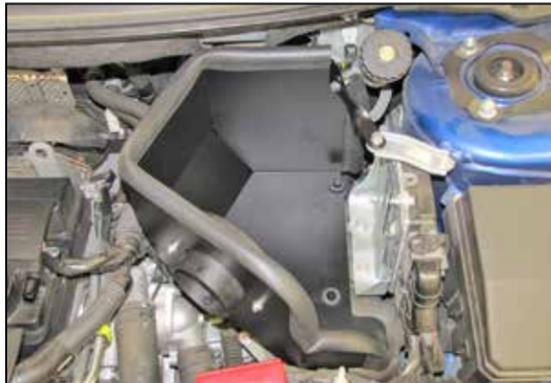
13. Install the heat shield assembly so the grommets engage the factory mounting studs, align the bracket with the ECU mount, install the provided spacer and secure with the provided hardware.
