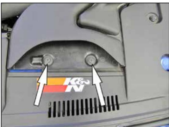
2. Remove the two plastic screws that secure the fresh air intake scoop to the core support and then lift up and remove the fresh air intake scoop from the vehicle.
