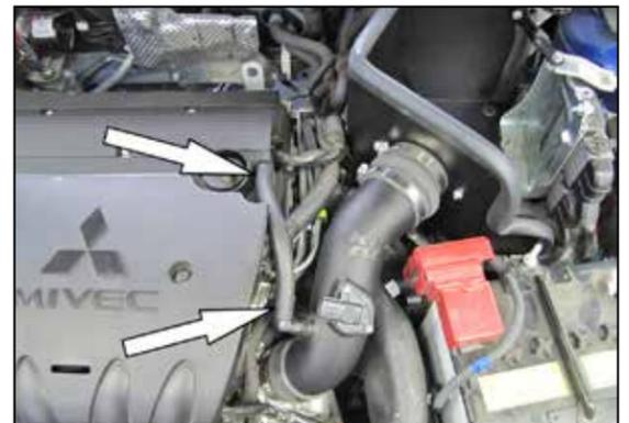
21. Install the provided crank case vent hose onto the fitting in the intake tube and then onto the fitting on the valve cover.
