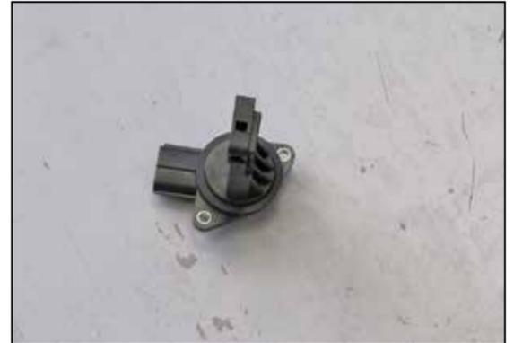
18. Install the provided gasket onto the mass air sensor.
