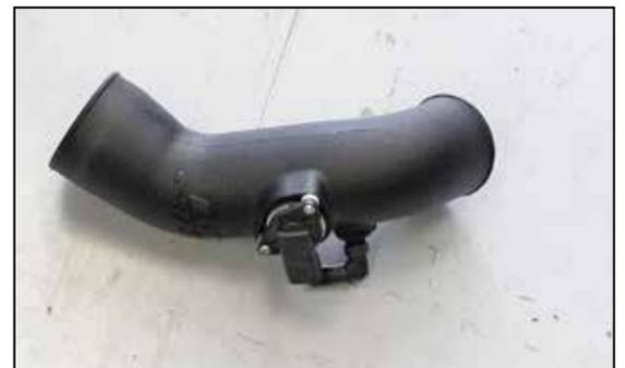
19. Using the four provided washers, install the mass air sensor into the K&N® intake tube and secure with the provided hardware.
