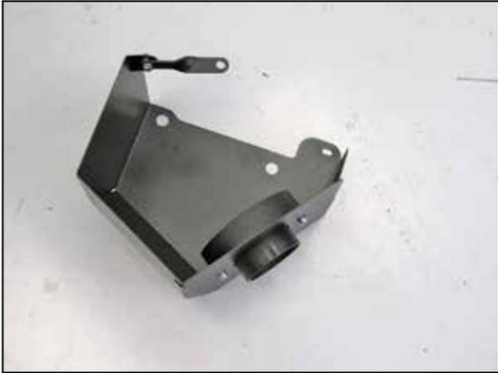
8. Install the heat shield mounting bracket onto the heat shield as shown and secure with the provided hardware.
