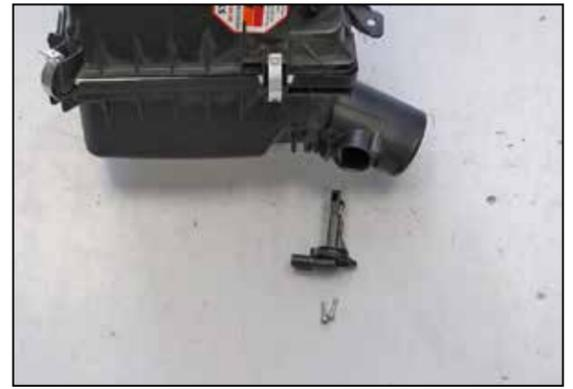
17. Remove the mass air sensor from the factory air filter housing.
