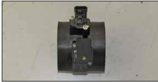
14. Install the sensors into the K&N® Mass air sensor housing and secure with the provided hardware.
