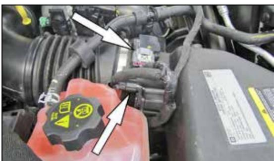
2. Disconnect the mass air sensor and humidity sensor electrical connections.
