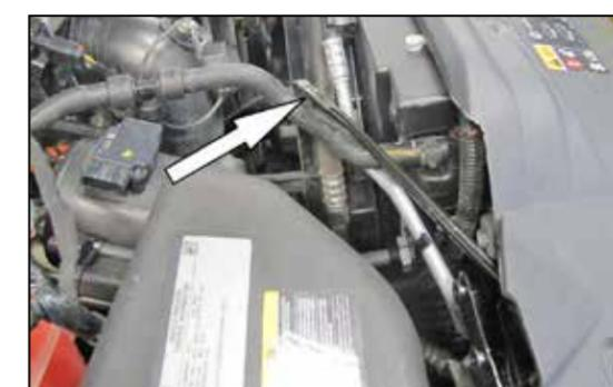
5. Loosen the bolt securing the fender brace to the core support then swing the brace clockwise towards the radiator for clearance.
