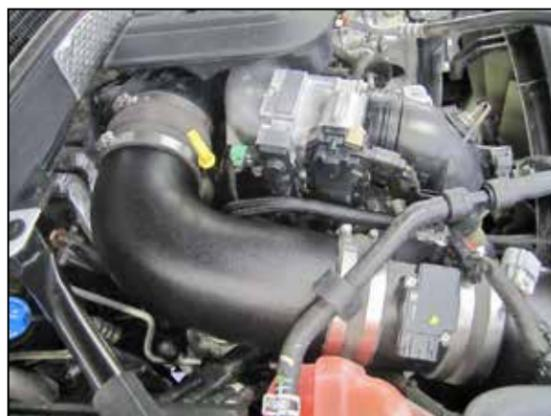
18. Install the K&N® intake tube into the hose at the Mass air sensor and then into the hose at the turbo inlet, adjust the tubes for best fit and then secure with the provided hose clamps.
