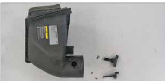
13. Remove the screws securing the Mass air sensor and Humidity sensor into the factory air box and then remove the sensors.
