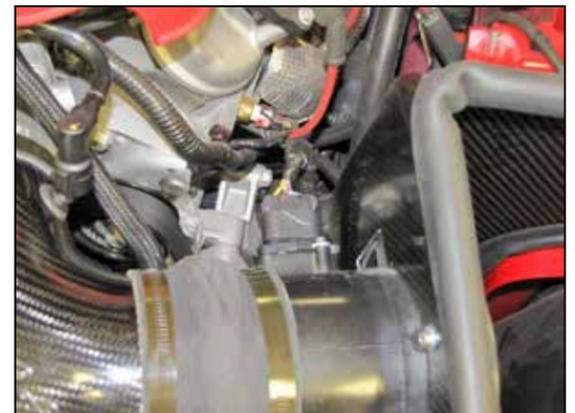
21. Reconnect the mass air sensor electrical connection.
