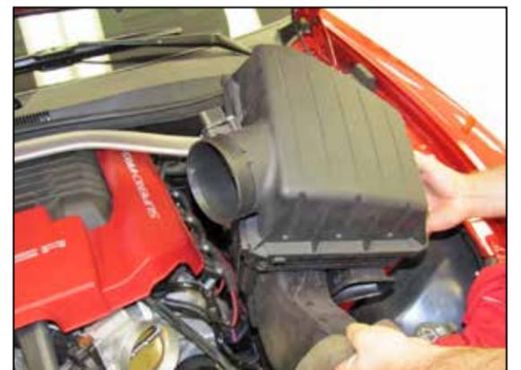
6. Remove the air box from the vehicle.
