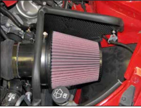
22. Install the K&N® air filter and secure with the provided hose clamp.
