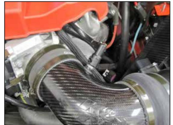
20. Rotate the crank case vent fitting clockwise and then connect to the fitting installed into the K&N® intake tube in the previous step.
