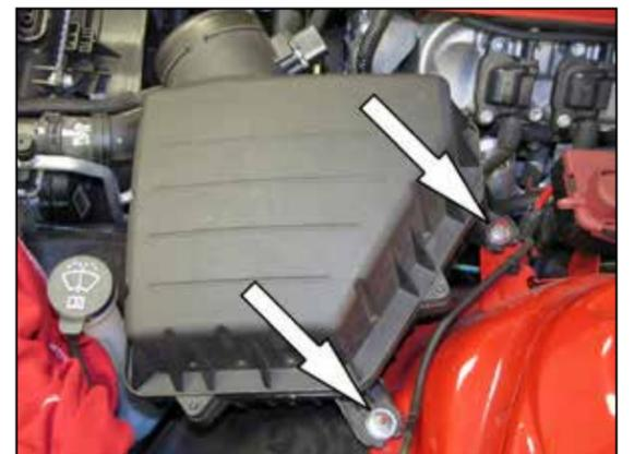
5. Remove the two air box mounting nuts shown.
