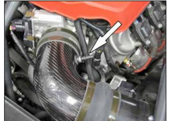
19. Install the provided crank case vent fitting into grommet in the K&N® intake tube as shown.
