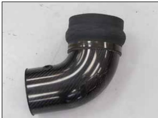
16. Install the provided hump hose (08695) onto the K&N® intake tube and secure with the provided hose clamp.
