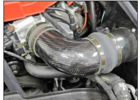
18. Install the K&N® intake tube assembly into the silicone hose at the throttle body and then install the hump hose onto the mass air sensor housing. Secure the tube with the provided hose clamps.
