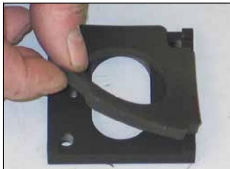
18. Peel the backing paper off and then install the provided gasket onto the K&N® mass air sensor adapter as shown.
