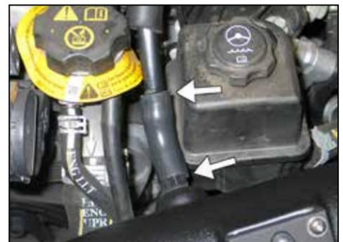
23. Install the provided crank case vent hose onto the factory crank case vent tube and then attach the open end to the vent fitting installed into the K&N® intake tube.
