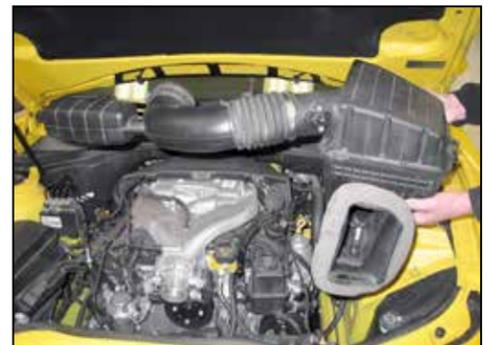
7. Remove the factory air box assembly from the vehicle.
