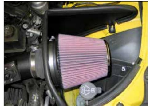
24. Install the K&N® air filter onto the filter adapter and secure with the provided hose clamp.
