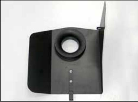
10. Install the filter adapter onto the heat shield and secure with the provided hardware.
