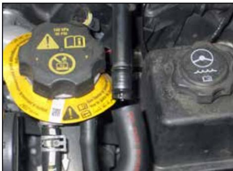
4. Disconnect the crank case vent hard line from the 90°connector hose on the factory intake tube.
