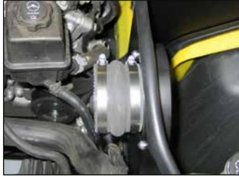
16. Install the provided silicone hump hose (08699) onto the filter adapter and secure with the provided hose clamp.
