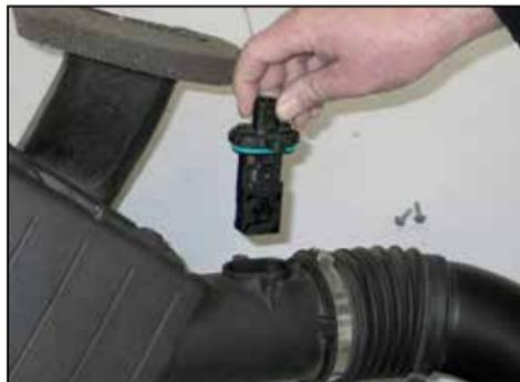
19. Remove the mass air sensor mounting screws and then remove the mass air sensor from the factory air box.
