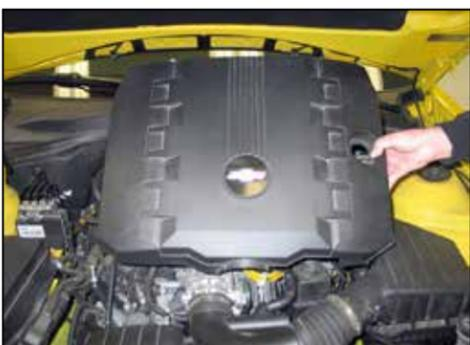
3. Remove the oil fill cap and then remove the engine cover from the engine. Reinstall the oil fill cap.
