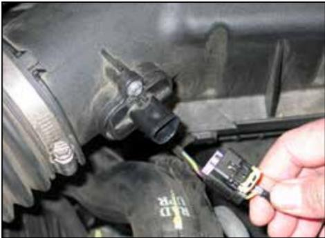
2. Release the locking and then disconnect the mass air sensor electrical connector.
