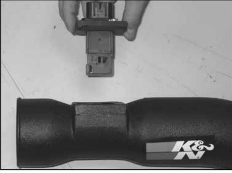
20. Install the mass air sensor assembly into the K&N® intake tube and secure it with the provided hardware.
