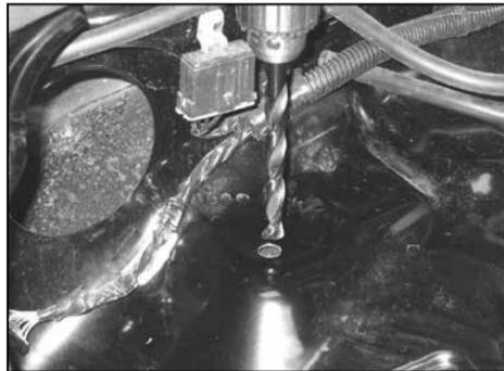
13a. On vehicles not equipped with the air box mounting stud and nut, drill out the existing hole in the inner fender with a 1/2" drill.
