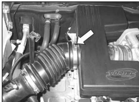
4. Loosen the hose clamp that secures the stock intake tube to the intake resonator.
