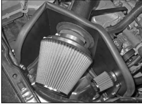
24. Install the air filter assembly onto the K&N® intake tube and secure with the provided hose clamp as shown.
