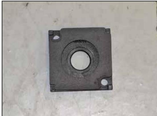
16. Install the provided gasket onto the temperature sensor adapter plate as shown.
