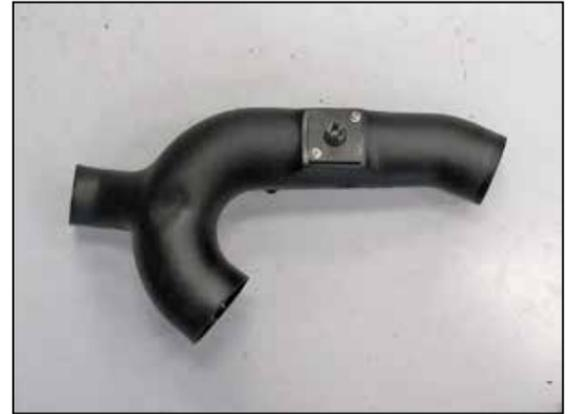
20. Install the inlet air temperature sensor assembly into the K&N® intake tube and secure with the provided hardware.
