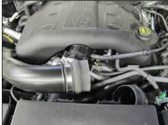
14. Install the provided hump coupler (087121) onto the passenger side turbo inlet tube and secure with the provided hose clamp.
