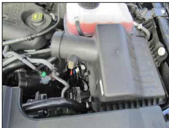
4. Release the three upper air filter housing retaining clips and then remove the upper air filter housing and factory air filter.
