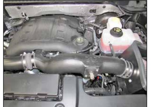
21. Install the K&N® intake tube into the coupling hoses and then secure with the provided hose clamps.
