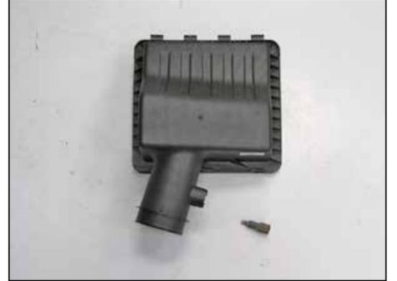
18. Remove the inlet air temperature sensor from the factory air filter housing.
