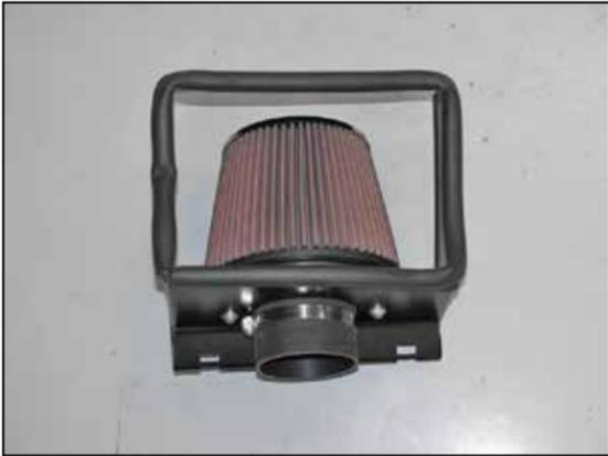
10. Install the provided coupling hose (08698) onto the filter adapter and secure with the provided hose clamp.
