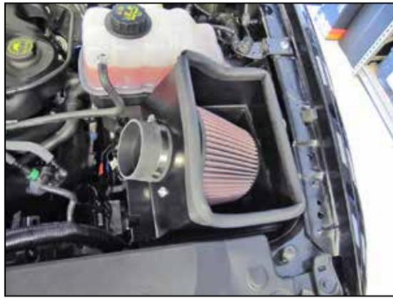
12. Install the heat shield assembly onto the lower air filter housing and secure with the factory retaining clip.
