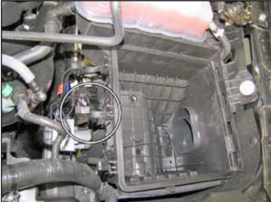
11. Remove the center upper air filter housing retaining clip as it will not be used.
