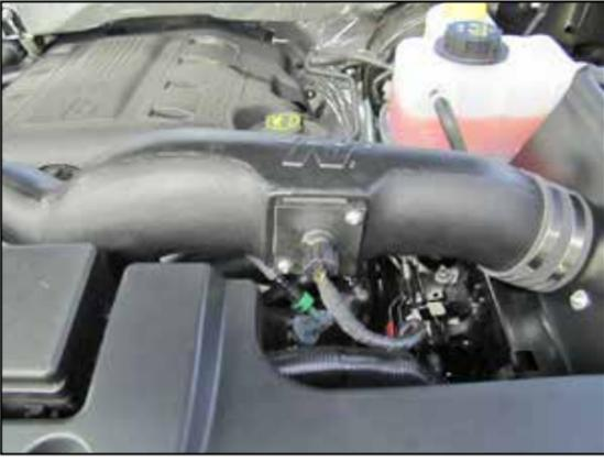
22. Connect the inlet air temperature sensor electrical connection.
