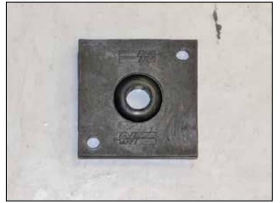
17. Install the provided gasket into the temperature sensor adapter as shown.
