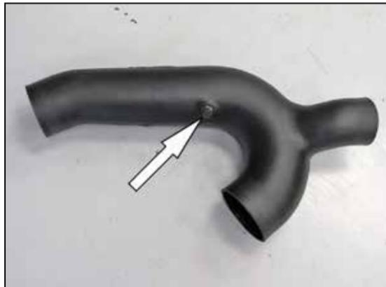
15. Install the provided 1/4"npt plug into the K&N® intake tube.
