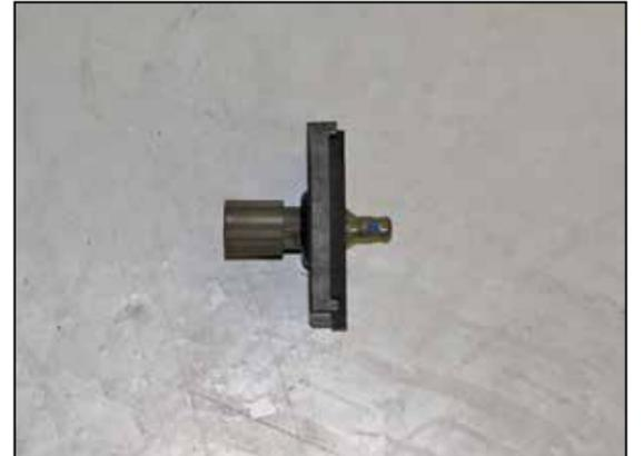
19. Remove the O-Ring from the sensor and then install the sensor into the grommet installed into the adapter as shown.
