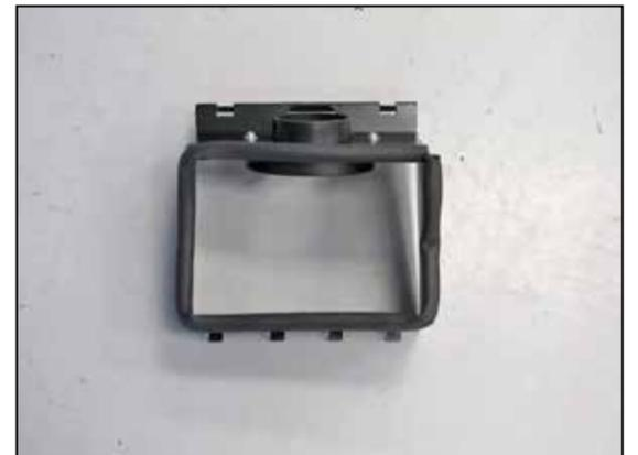
6. Install the "BULB" edge trim onto the top of the K&N® heat shield as shown.
