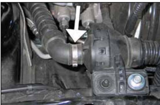
3. Cut the clamp that secures the engine pulse hose to the drum and disconnect the hose from the drum.
