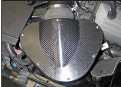
30. Install the K&N® airbox lid and secure with the provided hardware.
