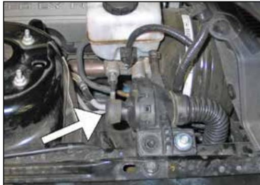
5. Install the provided cap onto the drum as shown.
