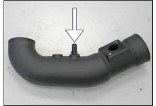
20. Install the crankcase vent fitting into the K&N® intake tube as shown.
