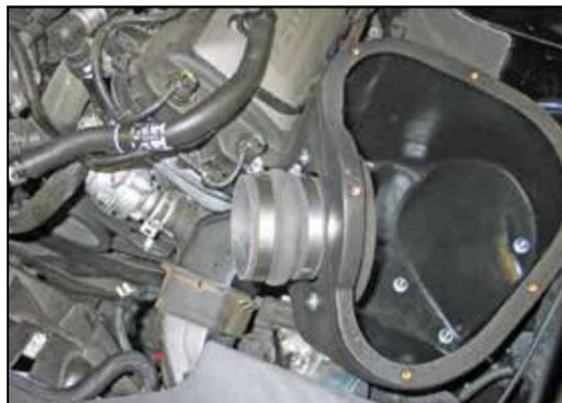
18. Install the provided silicone hose (08418) onto the filter adapter and secure with the provided hose clamp.
