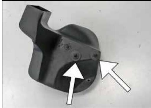
16. Install the airbox mounting grommets onto the two mounting studs installed on the K&N® airbox.
