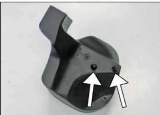
13. Install the two airbox mounting studs onto the bottom of the airbox and secure with the provided hardware.
