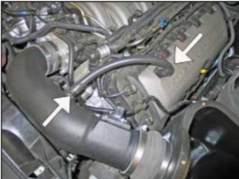
27. Install the crankcase vent hose to the fitting on the K&N® intake tube and onto the valve cover. Vehicles equipped with an EVAP vent line, connect it to the fitting installed in the K&N® intake tube.
