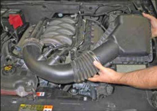
10. Remove the upper airbox and intake tube from the vehicle.
