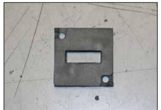
23. Install the provided mass air adapter gasket as shown.
