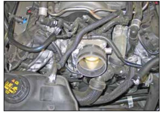
19. Install the provided silicone hose (08698) onto the throttle body and secure with the provided hose clamp.
