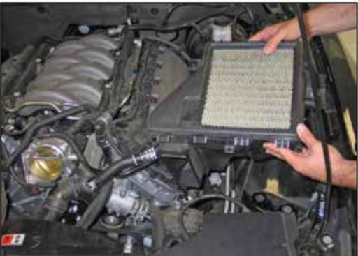
12. Remove the lower airbox from the vehicle.
