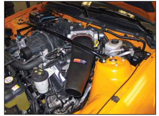
20. Install the K&N® intake tube into the throttle body and align with the mounting bracket, then secure with the provided hose clamp and hardware.
