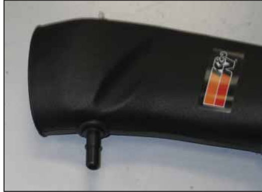
16. Install the factory crankcase vent fitting into the grommet installed into the K&N tube in step #14.
