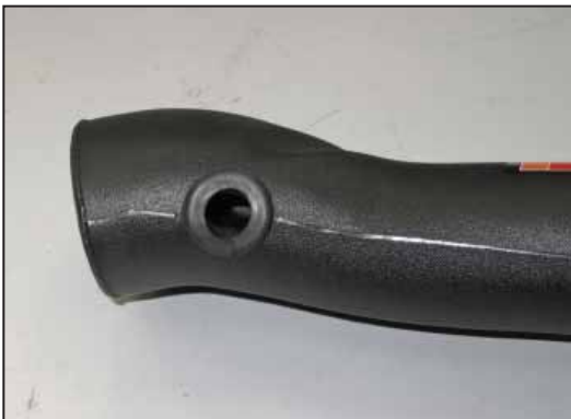
14. Install the supplied crankcase vent grommet into the K&N® intake tube as shown.
