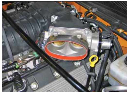
17. Install the supplied silicone hose (08627) onto the throttle body and secure with the provided hose clamp.
