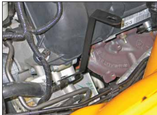
19. Install the tube mounting bracket (08761) onto the alternator bracket with the factory bolt removed in step #18.
