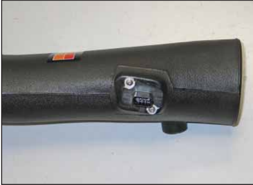
11. Install the mass air sensor into the K&N® intake tube and secure with the provided spacers and m4 bolts.
