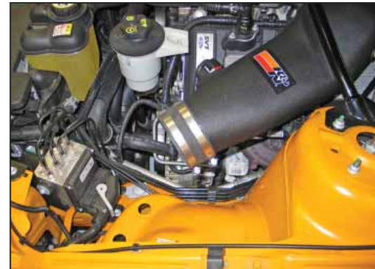
23. Install the silicone hose (08761) onto the intake tube and slide it past the bead on the end of the tube so proper clearance is maintained when the air filter assembly is installed.
