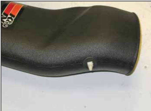
13. Insert the supplied 1/4" hose mender into the grommet that was installed in the previous step.
