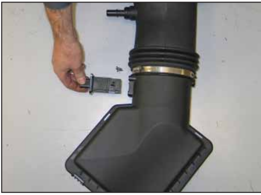
10. Using the provided T20 torx wrench, remove the mass air sensor retaining screws so the mass air sensor can be removed as shown.
