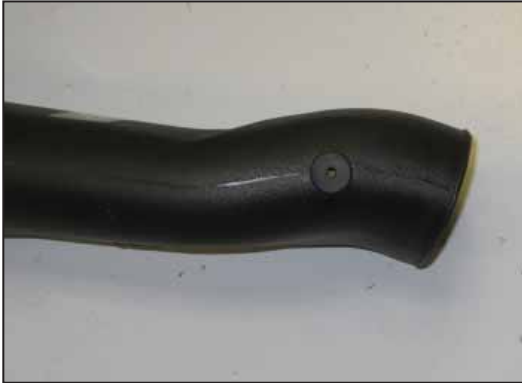
12. Install the supplied 1/4" id vent grommet into the K&N® intake tube as shown.
