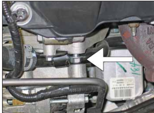
18. Remove the upper alternator mounting bolt shown
