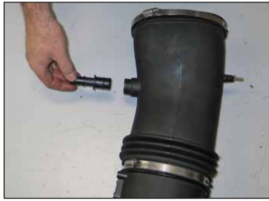
15. Cut the clamp securing the crankcase vent fitting into the factory intake tube and then remove the fitting from the intake tube as shown.
