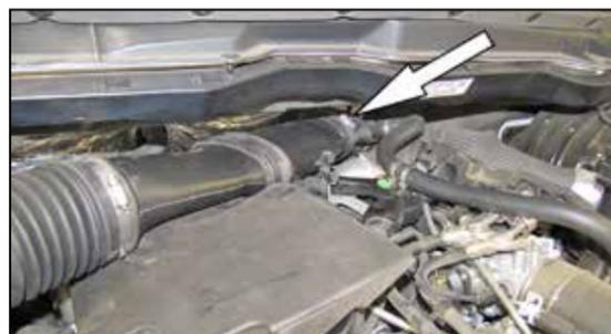
6. Loosen the hose clamp securing the intake tube to the turbo inlet hose. Lift up the intake tube to dislodge it from the mounting stud and then remove the tube from the vehicle.
