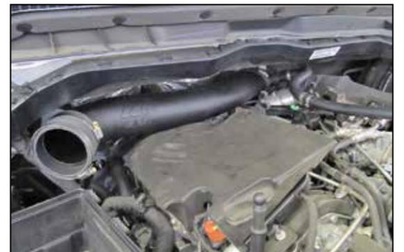
8. Install the K&N® intake tube into the factory turbo inlet hose and secure with the factory hose clamp.
