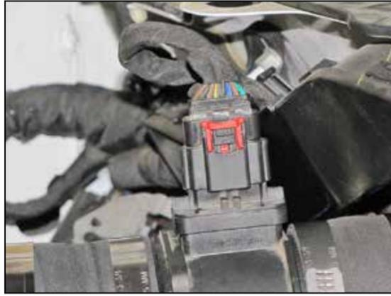
15. Reconnect the mass air sensor electrical connection.
