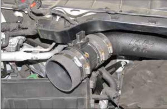
11. Install the mass air sensor into the coupling hose installed onto the K&N® intake tube.
