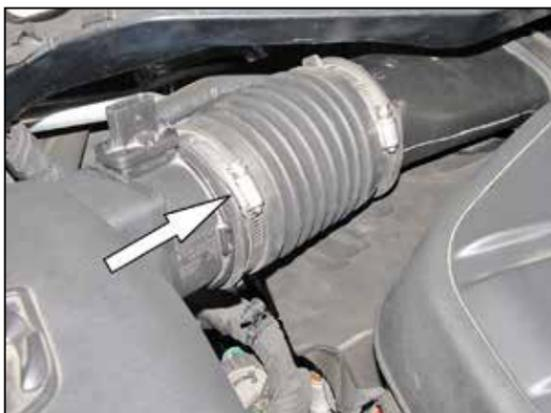
3. Loosen the hose clamp securing the factory intake tube to the mass air sensor.
