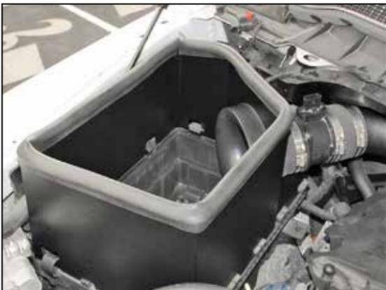
14. Install the heat shield onto the lower air filter housing and secure with the factory retaining clips.
