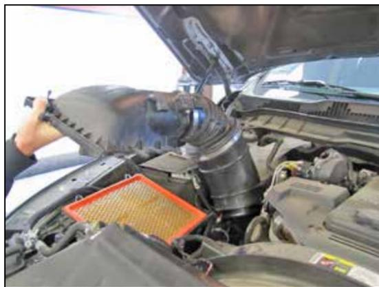
5. Remove air box lid and intake resonator from the vehicle.
