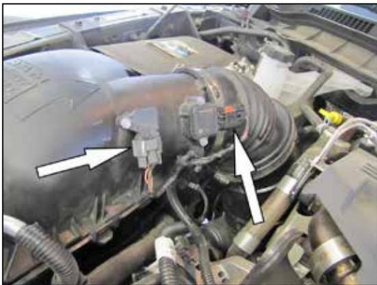
2. Disconnect mass air sensor and temperature sensor electrical connections, then unhook the wiring harness from air box.
