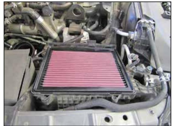
7. Install K&N® filter into air box base.
