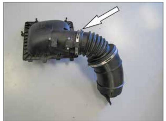
8. Loosen hose clamp securing intake resonator to air box lid and remove intake resonator from lid.
