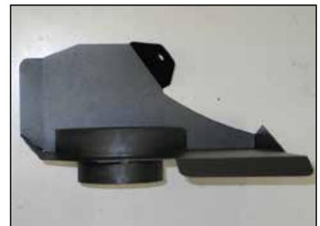
8. Install the filter adaptor into the heat shield and secure with the provided hardware.
