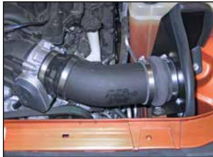
18. Install the K&N® intake tube into the silicone hump hose and then into the silicone step hose at the throttle body. Align the intake tube and heat shield for proper fit and then secure the intake tube with the provided hose clamps and the heat shield bracket with the factory air box retaining bolt removed in an earlier step.
