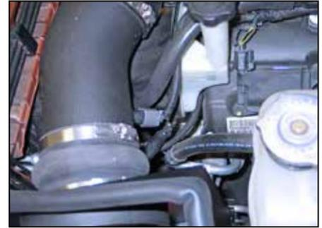
22. Reconnect the inlet air temperature sensor electrical connection.
