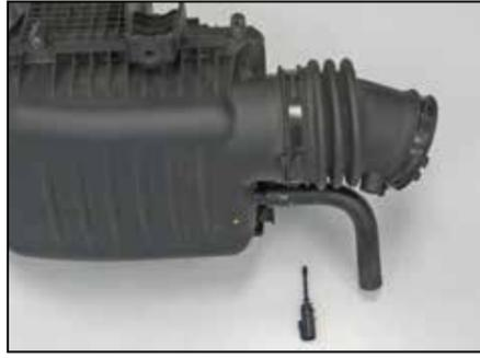
15. Remove the inlet air temperature sensor from the factory intake tube as shown.
