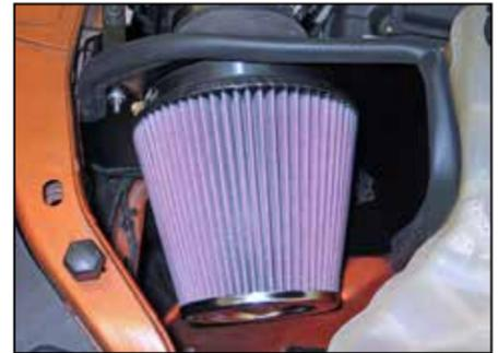
24. Install the K&N® air filter and secure with the provided hose clamp.
