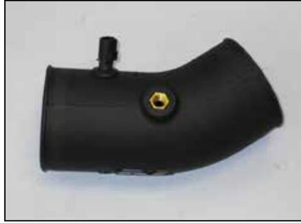
16. Install the provided grommet and the factory inlet air temperature sensor into the K&N® intake tube as shown.
