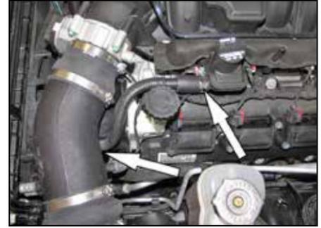
21. Install the assembled vent hose onto the fitting installed in the K&N® intake tube and then attach the open end to the valve cover port and secure with the provided hose clamp.
