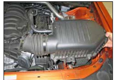
7. Lift up and remove the complete intake track from the vehicle.
