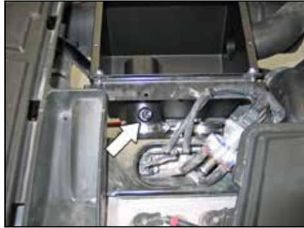
18. Install the provided npt vent fitting into the K&N® intake tube.
