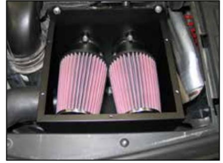
21. Install the K&N® air filters onto the intake tubes and secure with the provided hose clamps.
