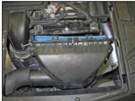
5. Depress the two locking tabs and then remove the air box half from the vehicle.
