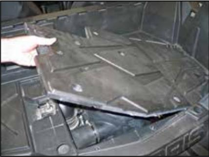
2. Remove the engine access panel from the cargo bay.
