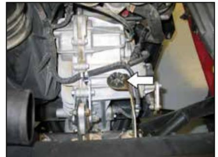
10. Remove the lower air box mounting grommet shown.
