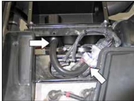
19. Install the provided idle by-pass hose onto the npt vent fitting and then onto the idle solenoid.
