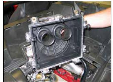
9. Remove the air box half from the vehicle as shown.
