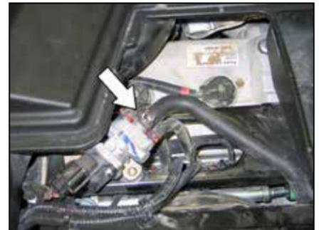
8. Loosen the hose clamp that secures the idle by-pass hose to the idle by-pass solenoid.
