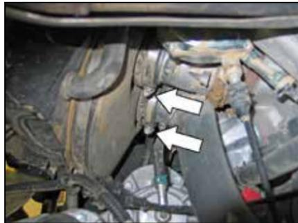
6. Loosen the two hose clamps securing the factory air horns to the throttle bodies.
