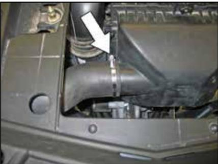
3. Loosen the hose clamp securing the fresh air intake hose to the air box and then disconnect the fresh air intake hose from the air box.
