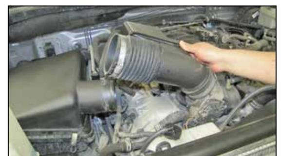
5. Remove the factory intake tube from the vehicle. **NOTE: K&N Engineering, Inc., recommends that customers do not discard factory air intake.**
