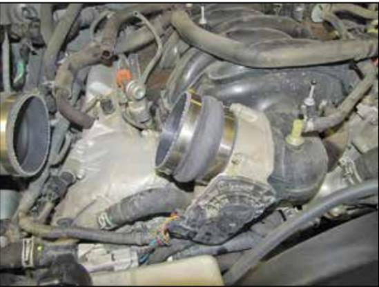
9. Install the provided hump coupling hose (08699) onto the throttle body and secure with the provided hose clamp.
