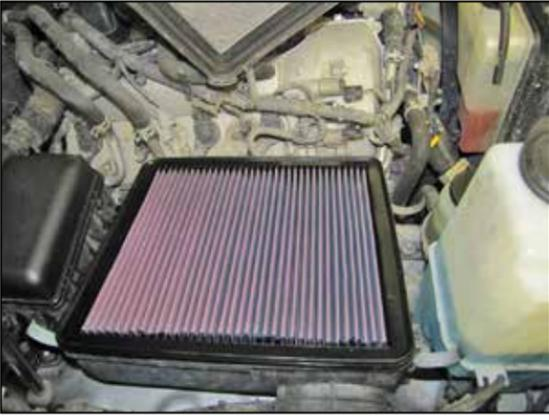
7. Install the K&N® air filter into the lower air filter housing and replace the upper housing but do not latch the retaining clips at this time.
