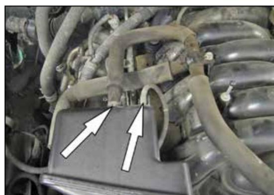
3. Disconnect the crank case vent hose and fuel pressure regulator vent hose from the factory intake tube.
