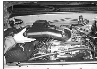
8. Remove the complete air induction system.
