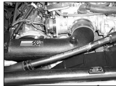
24. Install the K&N® intake tube onto the throttle body and secure with the provided hose clamp.
