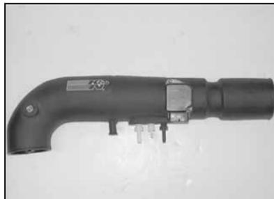
23. On 2000-02 models, install the three vents into the intake tube in the orientation as shown above.
