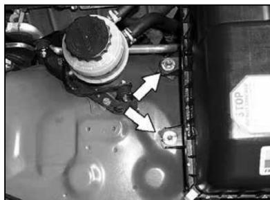
6. Loosen the three bolts that secure the air box assembly.
