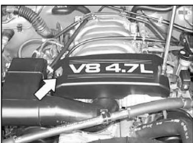
3. Loosen and remove the acorn nuts that secure the throttle body cover, then remove the cover.
