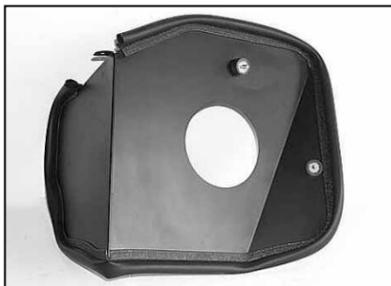
13. Install the two rubber mounted studs to the heat shield with the provided hardware, but do not tighten completely.
