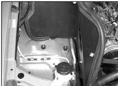
16. Install the heat shield onto the rubber mounted studs as shown above.
