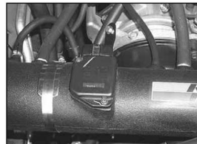
28. Attach the three provided, and one existing hose onto the K&N® intake tube as shown.
