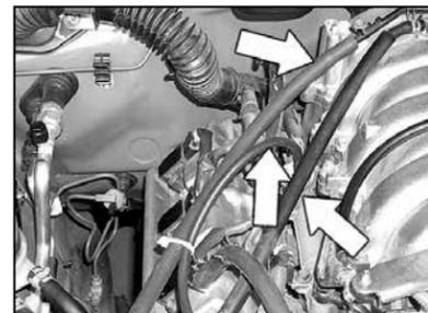
27. Install the three vent hoses onto the engine as shown above. (see arrows)
