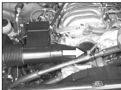
4. Loosen and remove the bolt that secures the AC line to the stock intake tube.
