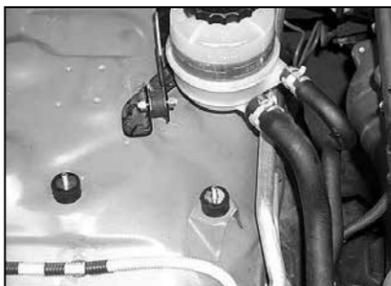
15. Install the two remaining rubber mounted studs to the original air box mounting holes.
