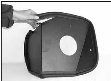
12. Apply the edge trim to the K&N® heat shield as shown above, trim if needed.
