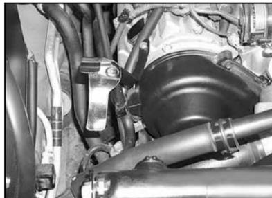
22. Install the saddle bracket assembly onto the existing threaded boss on the cam cover, do not tighten completely.
