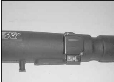
11. Install the mass-air sensor into the K&N® intake tube and secure with the provided spacers and screws as shown.
