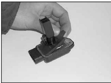
10. Apply the provided gasket to the mass-air sensor with the sticky side down.
