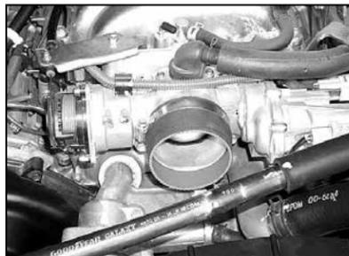
20. Install the silicon hose onto the throttle body and secure it with the provided hose clamp.
