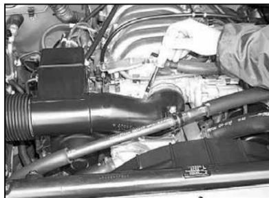
5. Loosen the hose clamp that secures the stock intake tube to the throttle body.
