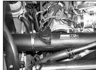
25. Secure the saddle bracket to the tube with the provided hose clamp.
