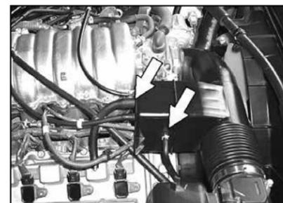
7. Disconnect the four rubber hoses from the engine as shown by the arrows.
