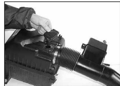
9. Loosen and remove the two screws that secure the mass-air sensor, then remove the mass air sensor.
