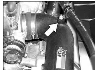
26. Re-connect the AC line to the K&N® intake tube using the original bolt.
