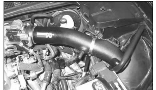
19. Install the K&N® intake tube assembly into the silicone hose at the throttle body and align with the saddle bracket installed in step #11. Secure the K&N® intake tube assembly with the provided hose clamps.
