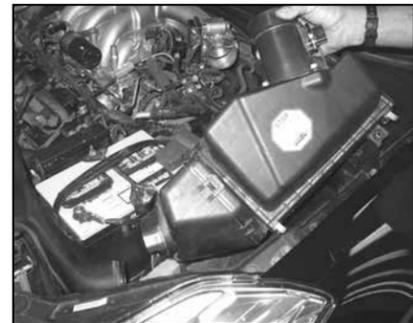
8. Lift the air box up from the mounting grommets. Detach the air box from the fresh air duct, then remove the air box from the vehicle.
