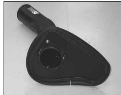
18. Secure the heat shield assembly to the K&N® intake tube with the provided hardware.
