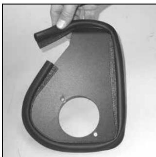
17. Install the provided edge trim onto the heat shield as shown.
