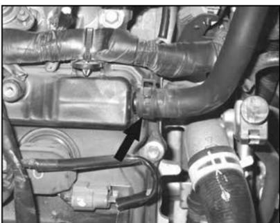
3. Release the spring clamp and disconnect the crank case vent hose.
