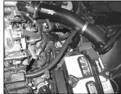
20. Install the provided crank case vent hose onto the vent port on the valve cover. Connect the open end to the 1/4" NPT fitting installed into the K&N® intake tube.
