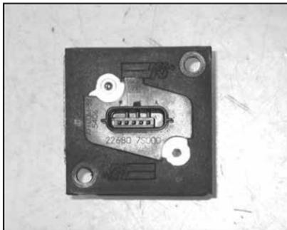
15. Install the mass air sensor into the K&N® mass air sensor adapter. Secure with the provided hardware.
