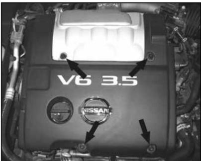
2. Remove the four bolts that retain the engine cover, then remove the engine cover from the engine.
