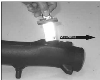
16. Install the mass air sensor assembly into the K&N® intake tube and secure with the provided hardware.
