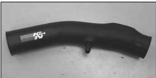
12. Install the 1/4" NPT fitting into the K&N® intake tube as shown.
