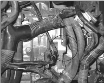
11. On 2004-2006 model vehicles, secure the tube mounting bracket assembly (06489) to the threaded boss on the transmission with the provided hardware.
