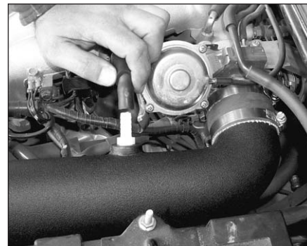
27. Reconnect the crank case vent onto the new K&N intake tube as shown.
