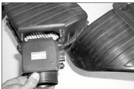
19. Remove the 4 nuts that retain the mass air sensor onto the factory air box then remove the mass air sensor as shown.
