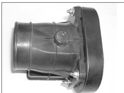
20. Install the K&N filter adaptor onto the mass air sensor with the hardware provided.
