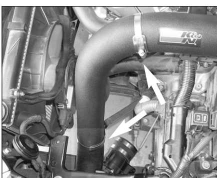
26. Line up the two saddle brackets onto the intake tube then secure the tube with the provided hose clamps.
