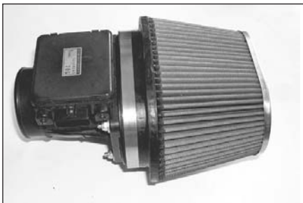
21. Install the new K&N filter charger onto the mass air sensor as shown.
