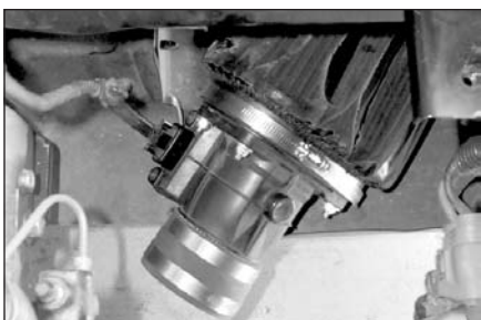
24. Reconnect the mass air sensor electrical connection then lay the mass air assembly on the inner splash pan as shown.
