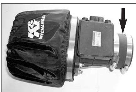
23. Install the silicone hose onto the mass air sensor with the provided hose clamps.
