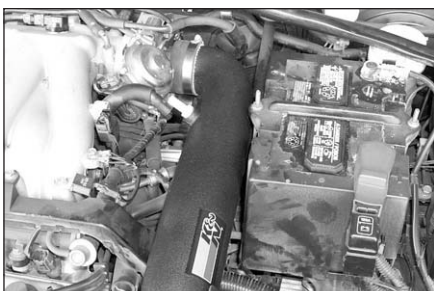
25. Install the new K&N intake tube onto the throttle body. Do not tighten hose clamps completely at this time.
