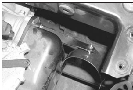
15b. Install saddle bracket assembly onto the transmission with the provided 10mm bolt. NOTE: make sure to install the provided spacer behind the new bracket.
