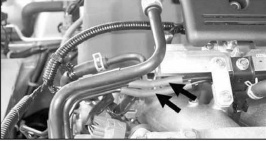
10. Detach the air control valve vacuum hose and the air control solenoid vacuum hose from the hard lines.
