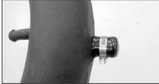
28a. On vehicles not equipped with an air injecting pump, install the provided "Caplug" onto the vent port on the K&N® intake tube and secure with the provided hose clamp as shown.
