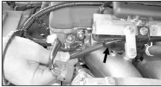
16. On vehicles equipped with air injection pump, attach the air control solenoid valve vacuum hose to the air control valve hard line. (lower hard line).
