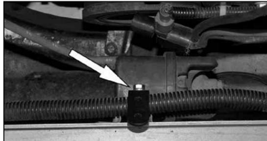
17b. Using the provided hardware, install the provided bracket (083155) along with the provided spacer and the factory vacuum canister.
