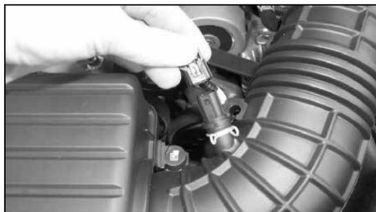
4a. On vehicles equipped with an air temperature sensor, disconnect the air temperature sensor electrical connection as shown.
