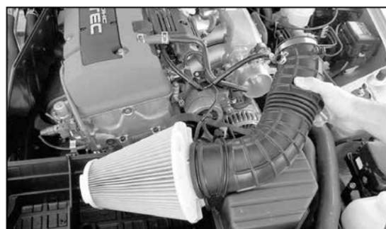
5. Loosen the hose clamp at the throttle body, then, remove the stock intake tube.
