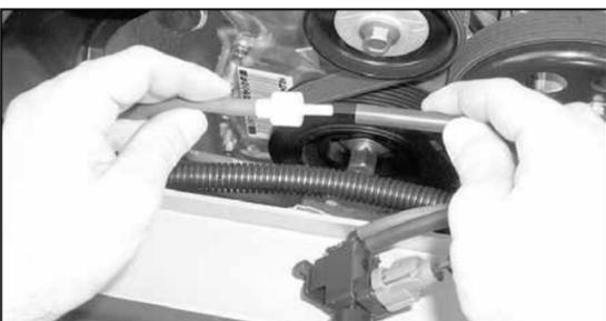
15. On vehicles equipped with air injection pump, attach the provided 4mm (short) vacuum hose to the check valve.
