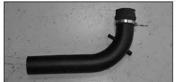
25. Install the silicone hump hose with provided hose clamps, onto the K&N® intake tube as shown.
