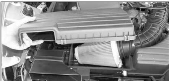
2. Release the 6 clips that retain the air box top, then remove the top.
