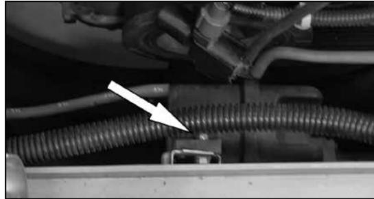
17a. Remove the bolt shown that secures the vacuum canister to the chassis.
