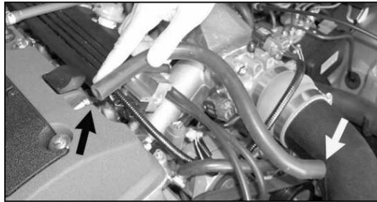
29. Attach the provided 1/2" hose to the crank case vent on the cam cover, then attach the other end to the vent on the K&N® intake tube.
