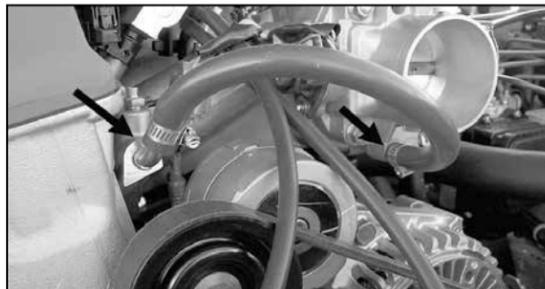
18. Attach the provided 1/4" reinforced hose to the fitting on the intake manifold and the fitting on the underside of the throttle body.
