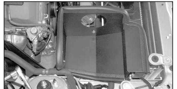
24. Using the provided hardware, install the heat shield assembly and secure the brackets to the original air box mounting locations.
