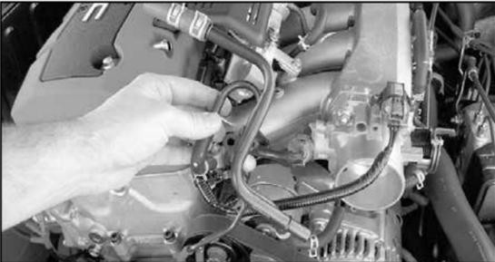
13. Remove the pipe assembly.
