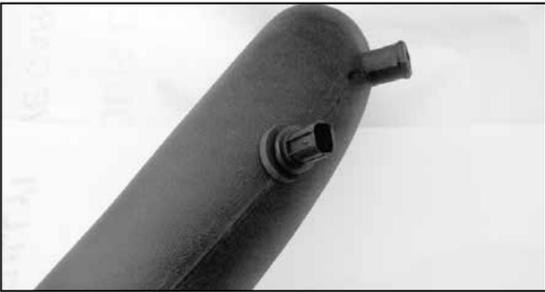
26c. Remove the air temperature sensor from the stock intake tube and install it into the grommet installed in the K&N® intake tube in the previous step as shown.
