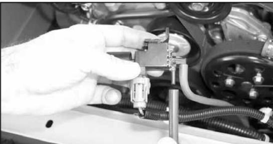
14. On vehicles equipped with air injection pump, attach the provided 4mm (long) vacuum hose to the air control solenoid valve.
