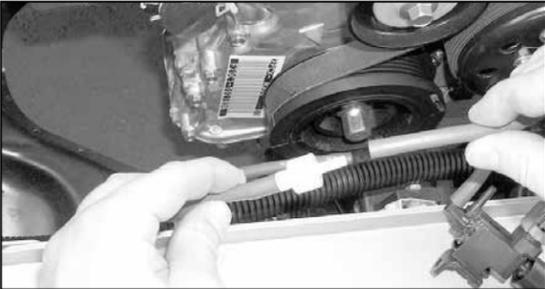
12. On vehicles equipped with air injection pump, detach the vacuum hose from the air control vacuum check valve.
