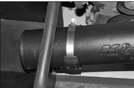
27. Install the K&N® intake tube onto the throttle body and align it with the saddle clamp on the heat shield and secure with the provided hose clamps.
