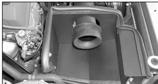
32. Install the radiused adapter onto the K&N® intake tube.
