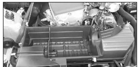
6. On vehicles equipped with air control solenoid, loosen and remove the screw and push clip that secures the air control solenoid valve to the air box base.
