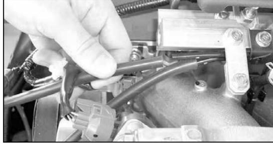
17. On vehicles equipped with air injection pump, attach the check valve vacuum line to the check valve hard line (upper hard line).
