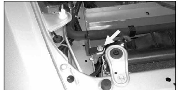
23. Using the provided hardware, install the small "L" bracket onto the vehicle as shown.
