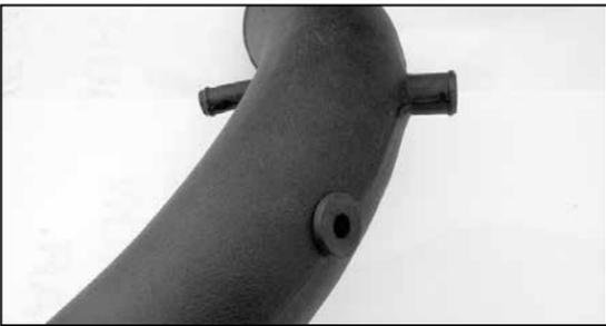
26b. On vehicles equipped with an inlet air temperature sensor, remove the intake tube from the vehicle and drill a 5/8" id hole at the spot indicated in the previous step. Install the provided grommet into the hole as shown.
