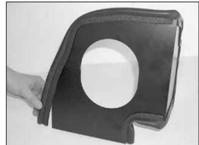
9. Apply the provided trim seal to the heat shield assembly as show.
