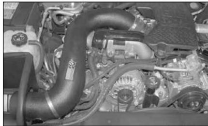
16. Secure the K&N intake tube to the intake manifold with the provided hose clamp.
