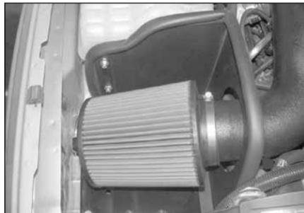
21. Install the K&N air filter onto the intake tube as shown and tighten completely.
