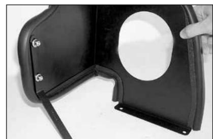
10. Install bracket onto heat shield as shown. Do not tighten completely.
