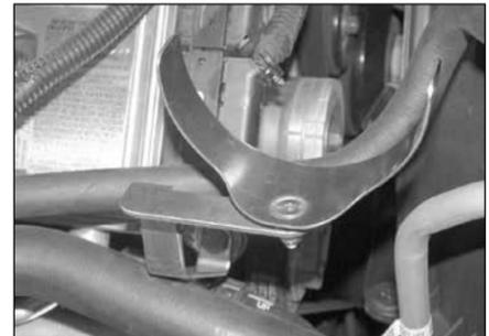
8. Using the factory bolt removed in step #7, install the tube-mounting bracket to the engine processor.
