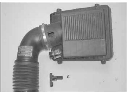
13. Using the "TORX" T20 wrench provided, loosen and remove the two-torx screw that retain the mass air sensor, and then remove the sensor.
