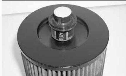
20. Install filter restriction gauge onto K&N air filter as shown.
