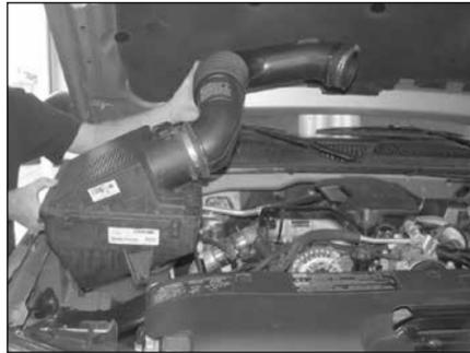
4. Lift up on the air box assembly to release from the mounting grommets, and then remove the air box and intake tube assembly from the vehicle.
