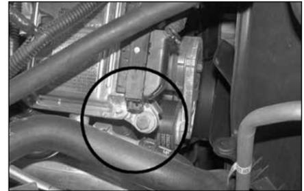
7. Remove the lower front engine processor mounting bolt shown.
