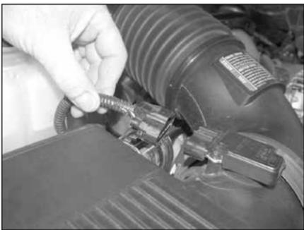
2. Depress the locking tab on the mass air sensor electrical connector, and then disconnect the electrical connection.
