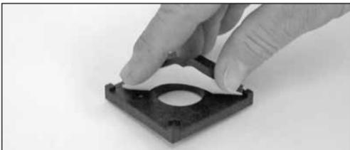
15. Install the provided gasket onto the mass air sensor adapter as shown.
