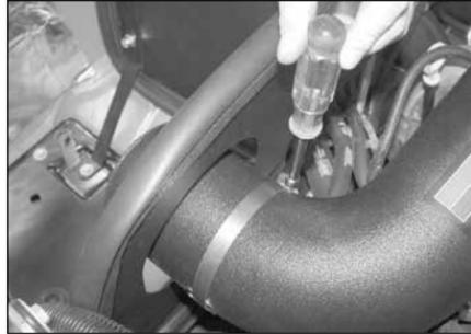
17. Install saddle bracket onto intake tube with hose clamp provided. Adjust for best fit and tighten all hardware.
