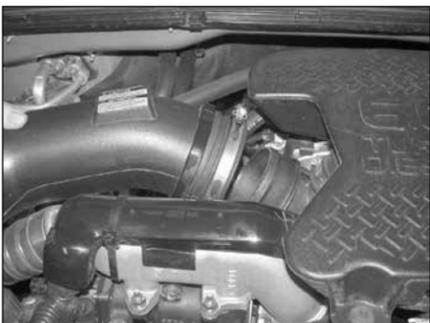
3. Loosen the hose clamp, which secures the intake tube to the intake manifold, and then disconnect the intake tube from the intake manifold.
