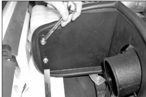
18. Adjust heat shield and bracket for necessary clearance, then tighten all hardware completely.
