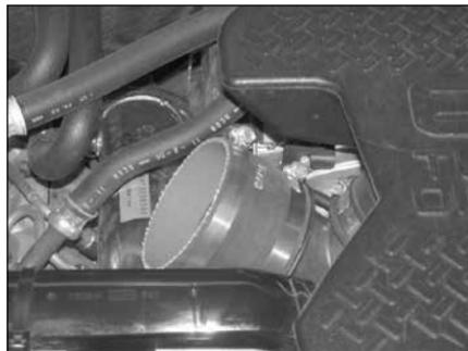
5. Install the silicone hose (08456) onto the intake manifold and secure with the provided hose clamps.
