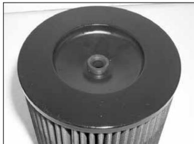
19. Install grommet onto filter as shown.
